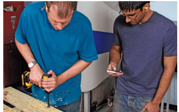
Speed drills. In two other tests, they recorded how fast each tool could drill 10 1-in.-dia. holes through a 4x4 post, and drive 50 more of the 3-in. screws.
