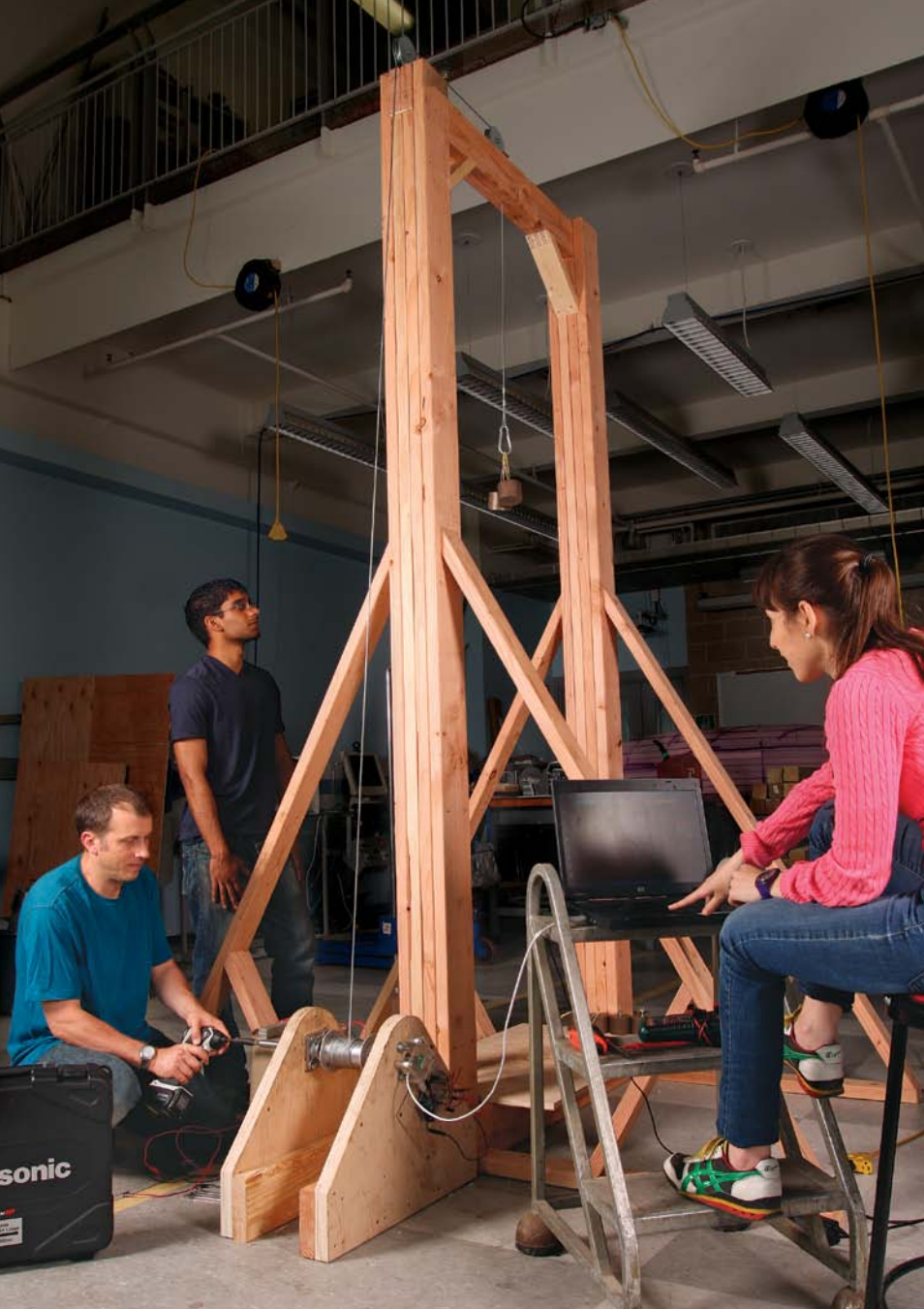
Up she rises. To gauge each drill's sustained torque, Constans and his students built the "guillotine" and used it to see how much weight the tool could lift.
