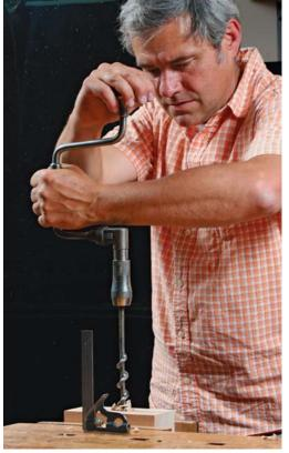
Clear the waste. Drill two ¾-in. holes on your centerlines. Go halfway, flip the piece, and finish from the other side. Use a square as a visual aid to keep the bit straight.
