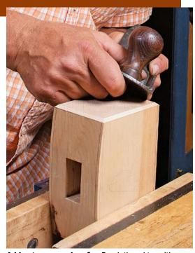
**Add a generous chamfer.** Break the edges with a handplane to help prevent splintering or chipping in use. Sand away the tool marks, if you like.
