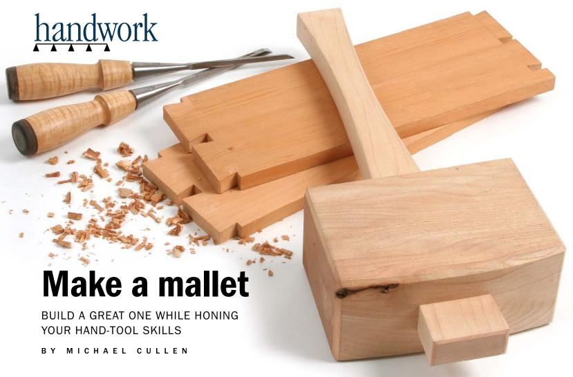
like a stout woodworking mallet with an oversize head. Why? It lets me generate plenty of force for cleaning out a mortise or chopping dovetails, and I can also use it for delicate detail work by just choking up on the handle.
