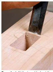
**Taper last.** At the top, chisel out the taper by working back toward the marked lines.
