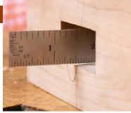
**Check for flatness.** A small rule reveals any bumps or hollows in the walls of the mortise.
