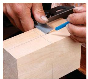
**Start with centerlines.** Mark them carefully and carry them around the head. Then lay out the ends of the mortise, plus the extra distance for the taper.
