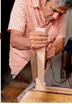
**Saw the tapers.** Make a small crosscut at the narrowest part of the handle and then saw down into it, keeping to the waste side of the line.
