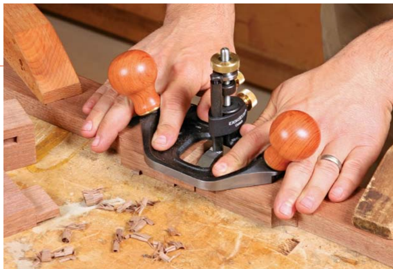
Lock in the setting with the depth collar. They're standard in big planes and let you raise the blade to take lighter shavings but still get back to the final depth.
