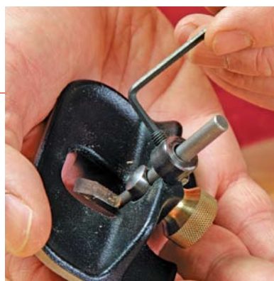
Lock in the depth. Because small planes don't come with collars, use a drill-bit stop collar to do the job. Now you can work down to the final depth.
