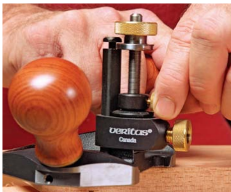
Lock in the setting with the depth collar. They're standard in big planes and let you raise the blade to take lighter shavings but still get back to the final depth.
