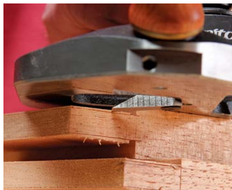
Set blade depth from a scribed line. Lower the blade until the cutting edge is aligned with the cut line left by a marking gauge.
