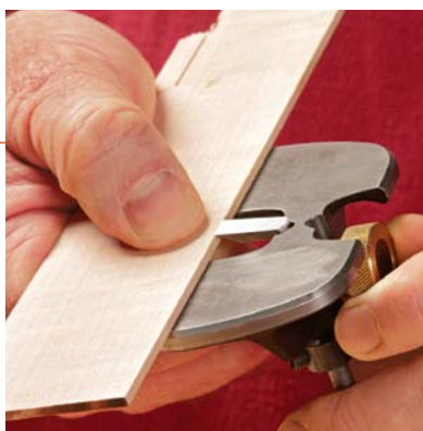
Use inlay to set depth. Set the blade just shy of the inlay's thickness. This leaves the inlay proud of the surface, so you can scrape and sand it flush.
