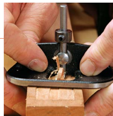
Support is important. The sole on both sides of the blade needs a surface to rest on, ensuring that it doesn't tip and plane an uneven bottom.
