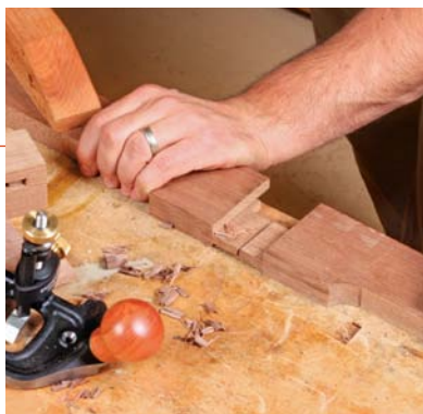
Get support on both sides of the blade. Set two rails end-to-end so that you can trim two tenons at once. With a large model, the sole is wide enough to bridge both tenons and rest on both rails (right).
