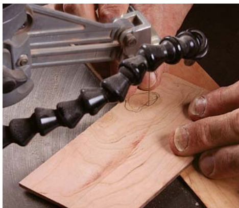
Find your patch. Use the transparent pattern to find a nice, tight knot of similar size on a piece of scrap and resaw it to about \frac{3}{16} in. thick. Draw a similar outline and cut it out on a scrollsaw.
