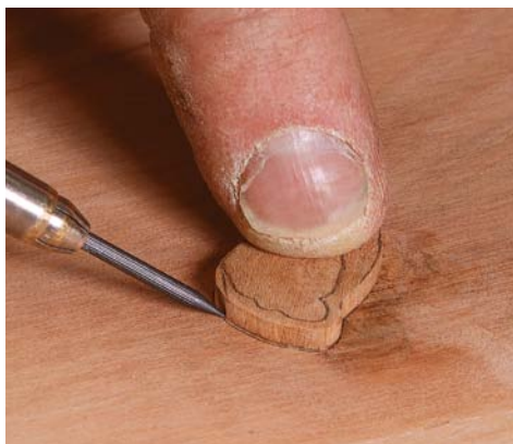
Draw around it. Place the patch so that it covers the whole knot and draw around it with a very sharp pencil.
