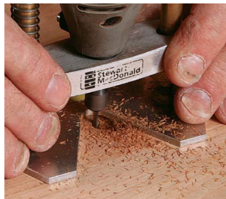
Make a recess. Use a small plunge router or a rotary tool in a plunge base to excavate to a depth of about \frac{1}{8} in. After that, work up to the layout lines with a small chisel or gouge.
