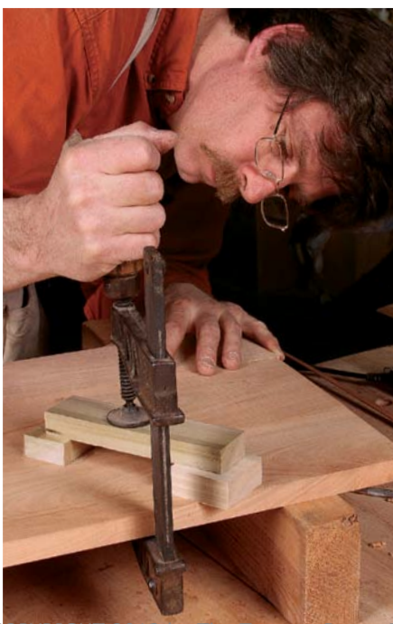
Find your patch. Use the transparent pattern to find a nice, tight knot of similar size on a piece of scrap and resaw it to about \frac{3}{16} in. thick. Draw a similar outline and cut it out on a scrollsaw.
