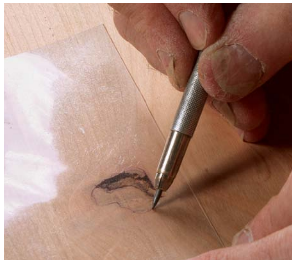
Trace the knot. Draw the outline of the loose knot on a piece of clear plastic, such as a three-ring file divider.
