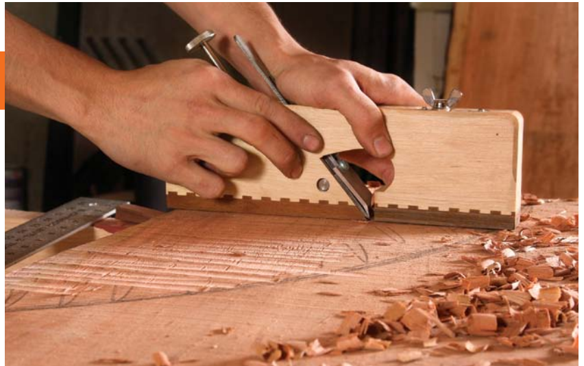
Level the high spots. The scrub plane is designed for heavy stock removal. It makes deep, fluted tracks and thick, brittle chips.
