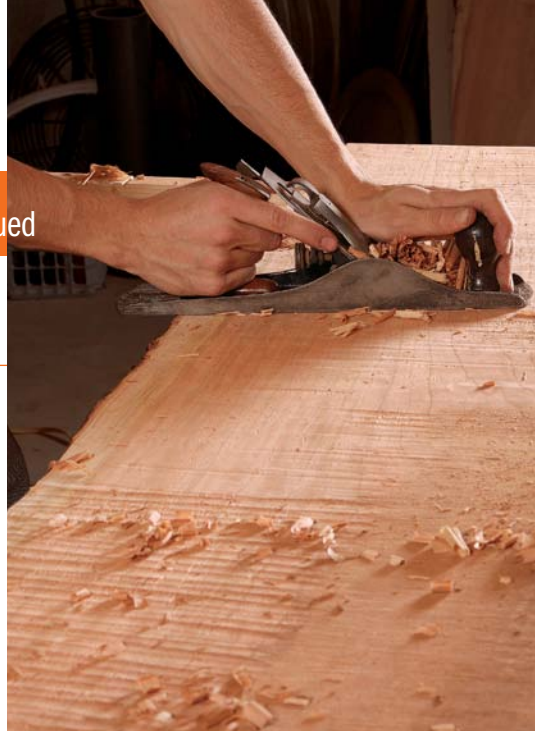
Refining the surface. The jack's wider, shallower cut levels the ridges left between the scrub plane's ruts. Work across the grain and diagonally.
