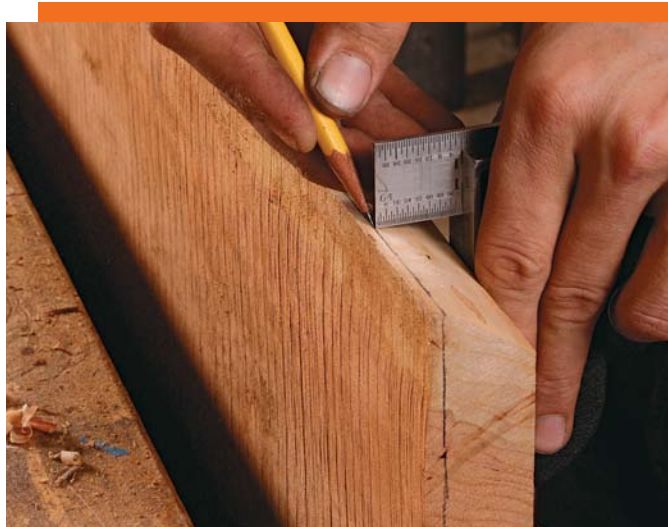
Mark out the thickness. Set a combination square to the desired thickness and reference from the flattened face to draw a line along all four edges.
