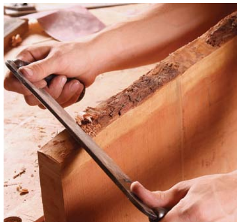
Use a drawknife to remove the bark. Short strokes and a shallow angle lift the bark without digging into the surface underneath.
