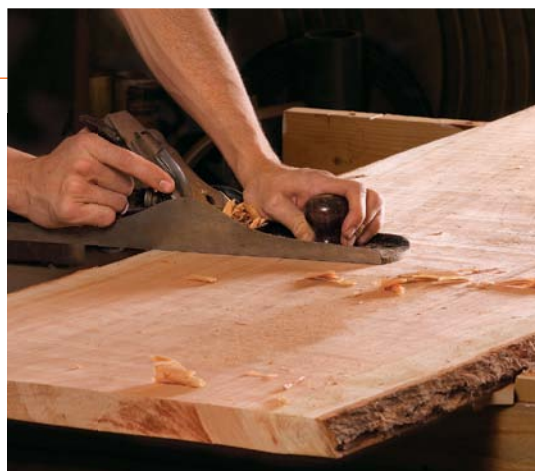
Start across the grain. Change directions as needed. The plane's long sole will find any remaining high spots, bridging the valleys that a shorter plane would follow and deepen.
