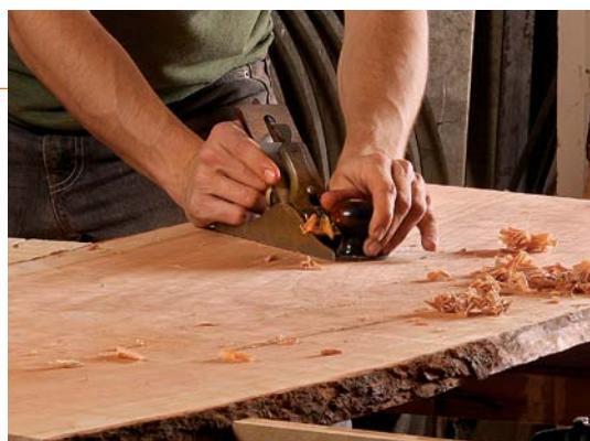
Tackle tearout. Working in all directions, remove whisper-thin layers from the entire slab until the tearout is trimmed away, leaving a dead-flat, glassy surface.
