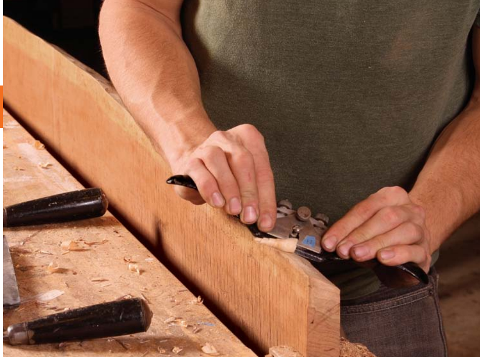
An irregular surface calls for a nimble tool. The spokeshave's short sole leaves the contours of the edge intact while shaving the surface smooth.
