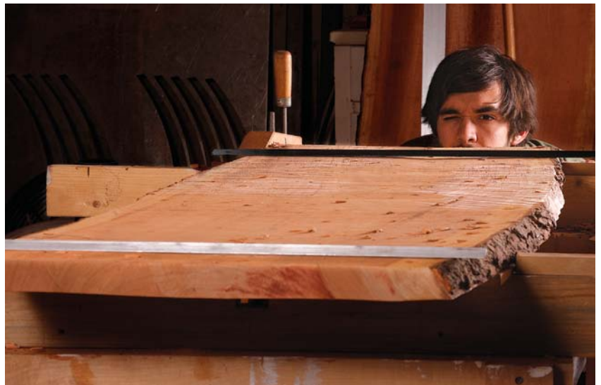
Check your progress with the straightedge. There is no reference line against which to gauge your work, so you'll need to take repeated sightings with the winding sticks and long straightedge.
