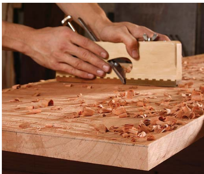
Flip the board and repeat the process. Stay with the scrub plane for quick stock removal until you get close to the layout lines.
