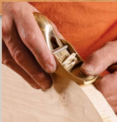
Edges This versatile tool should also be able to smooth both straight and curved edges.
