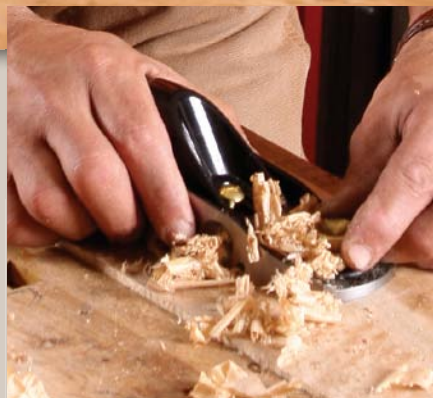
Face grain With a tight mouth and sharp blade, you should be able to handle a curly hardwood.
