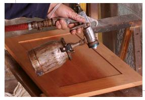
Pad on small surfaces or spray like a pro. Although vinyl sealer is designed to be sprayed (left), you can pad it on if you work quickly and in small areas (above). Vinyl sealer is ideal under solvent lacquer and two-part catalyzed finishes. The main drawback is the fumes, so wear a respirator when spraying or working with poor ventilation.
