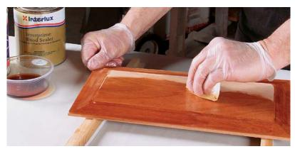
**Avoid shellac.** Shellac is too brittle to use as an exterior sealer and will fail with severe wood movement, so you can either thin the varnish topcoat by 50% with mineral spirits, or use a marine-grade sealer that doesn't contain stearates.
