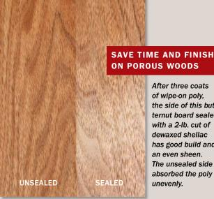
After three coats of wipe-on poly. the side of this butternut board sealed with a 2-lb. cut of dewaxed shellac has good build and an even sheen. The unsealed side absorbed the poly unevenly.
