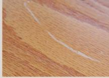
A flaky finish. On this window seat, a waterborne topcoat was applied over a stearated sealer. The weak bond between the two types of finish caused the topcoat to delaminate after it was scratched.
