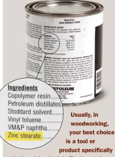
designed for the job. That's not the case with many products sold as "sanding sealers," whether waterborne or oil-based. The latter consist of a vinyl-alkyd resin that seals, a fast-drying solvent such as toluene that allows you to recoat in under an hour, and zinc stearates or metallic soaps to make sanding easier. These last components are the sealers' Achilles heel. They make the sealer soft and tend to produce a weak bond with the substrate and subsequent coatings.
