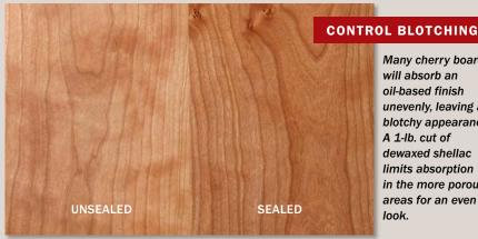
Many cherry boards will absorb an oil-based finish unevenly, leaving a blotchy appearance. A 1-lb. cut of dewaxed shellac limits absorption in the more porous areas for an even look.
