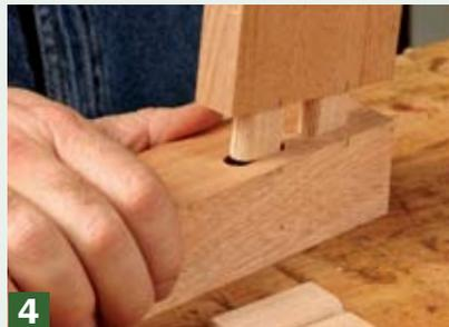
**4** **Insert the tenons and assemble the joint.** You'll get a perfect fit in minutes.
