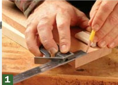
**1** **Mark the center of the mortise.** As with a biscuit joiner, these marks will guide the tool.
