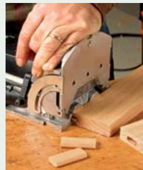
**Simple, precise setup.** A movable fence (left) has detents at common angles and a series of vertical stops. Alignment pins on the front of the tool (right) locate mortises a set distance from the end or edge of a workpiece.
