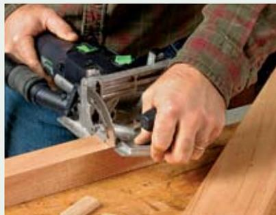
**3** **Hold steady and plunge slowly.** Align the center mark on the fence with the mark on the workpiece.
