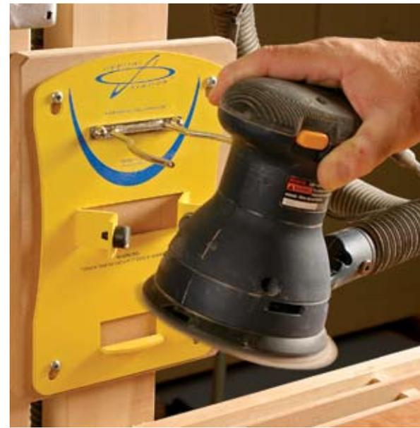
**Adjustable yoke holds most random-orbit sanders.** The upper portion of the sander slips into the yoke while the bottom end of the sander rests against a pair of rubber bumpers.
