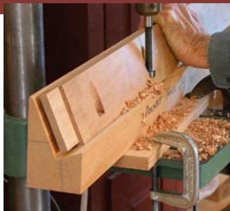
**Jig simplifies pocket-hole drilling.** A shop-made drill-press jig holds the apron at a suitable angle for drilling the pocket holes with a Forstner bit (above). A screw driven through an oversize shank hole in the pocket joins the top to the apron (right) while allowing the top to expand and contract.
