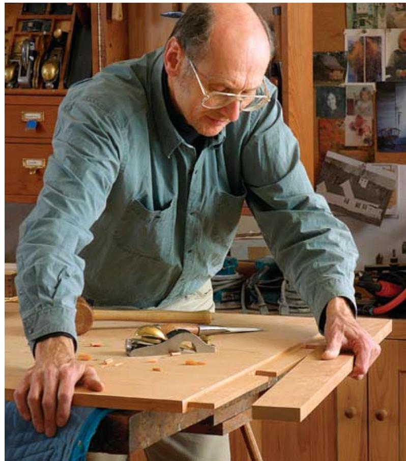
**Assemble the breadboard ends.** Check the tenon fit in the breadboard mortise, and trim the tenons as needed. When the fit is right, use pipe clamps to snug the breadboard ends to the tenon shoulders, then drill holes all the way through for the pins.
