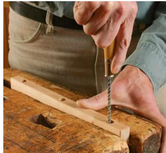
**Elongate the end holes.** A typical cleat has three holes, with the two nearest the ends elongated to allow the top to expand. The author uses a round rasp for the job.
