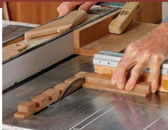
**Make the buttons.** After rabbeting the end of a board to create a lip, Becksvoort uses a tablesaw and a miter gauge to crosscut the stock into individual buttons.
