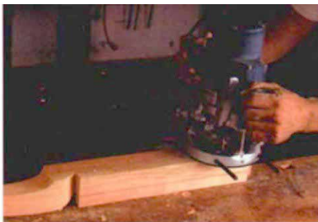
A plunge router with a spiral bit roughs out the mortises. The full stock width of the blank provides support for the router.
