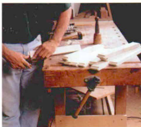
Mark the shoulder line on the narrow edge of each tenon. Cut the waste away on the handsaw.
