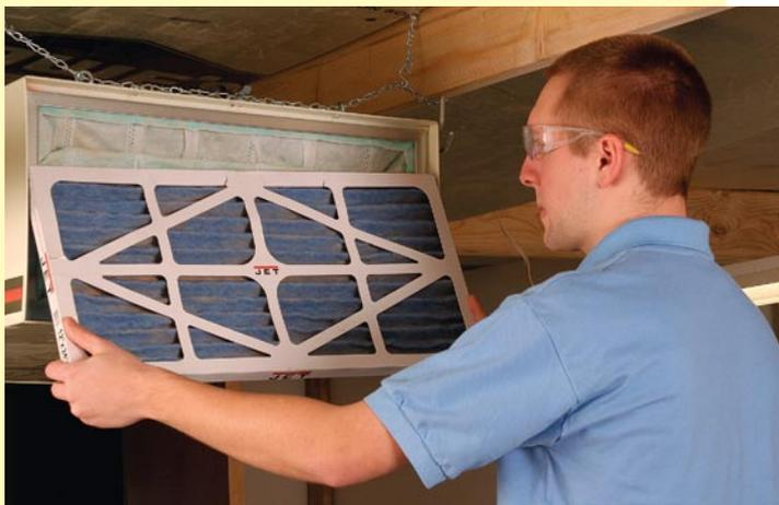
**Two-stage filtering.** The outer filter traps dust as small as 5 microns. This is the filter you'll change most often, but it is a standard size, available for under \$20. The inner filter collects dust down to 1 micron. It is more expensive, and available from the manufacturer.
