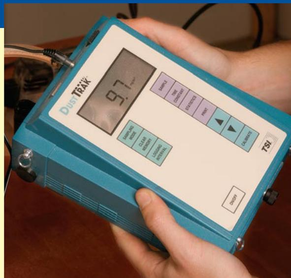
**Then turned on the meter.** The monitor used to track dust concentrations detects particles between 0.1 micron and 10 microns, so it provided an accurate reading of whether the filter was collecting the most harmful dust.
