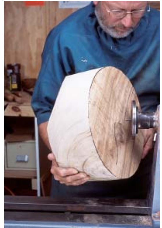
Heavy blanks are easiest to mount with the lathe running just fast enough to feed the screw into the center hole.
