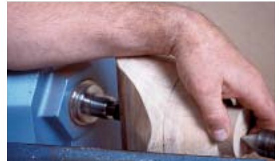
On blanks with a symmetrical round face, align the two-spur drive along the main axis of the curve on top of the blank. Mount the blank with the top at 90 degrees to the lathe axis and the sides evenly balanced. A pencil line drawn on the roughed bowl profile indicates how much the blank needs to be repositioned to bring the lower portions of the rim into the same plane (left, center). Make this adjustment easier by using the lathe to support your arm as you pivot the blank on the two-spur drive (above).
