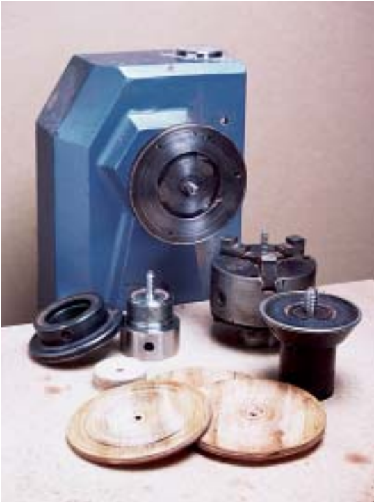
A range of screw chucks enables you to provide optimum support for a blank.
