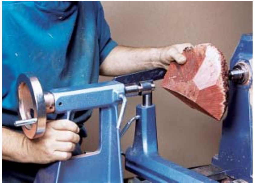
To mount a blank with an uneven surface between centers, chisel a V-groove to receive a two-spur drive (left). As you bring the tail center up, steady the blank by resting your arm on the tool rest (above).
