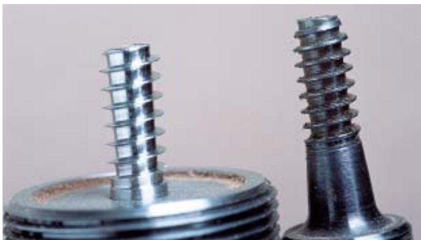
The Glaser screw (left) with its finely machined thread is vastly superior to the copy (right), typical of many offered as a chuck accessory.
