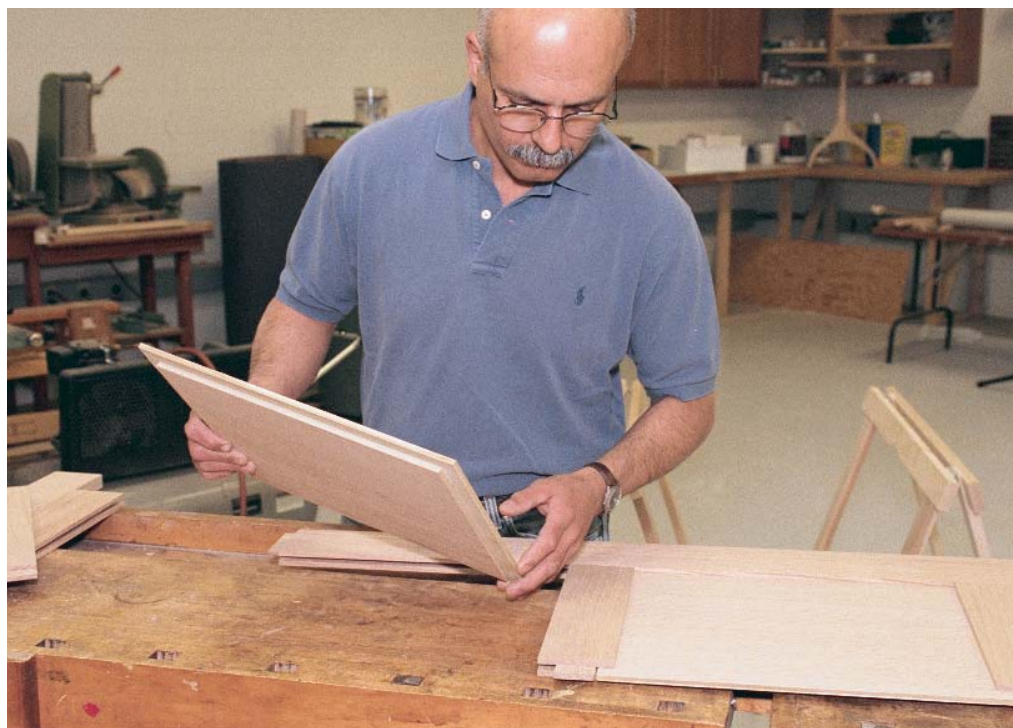
Fast rabbets with a dado blade. The panels are rabbeted with a dado blade. The frame-and-panel overmantel is glued up before it leaves the shop.
