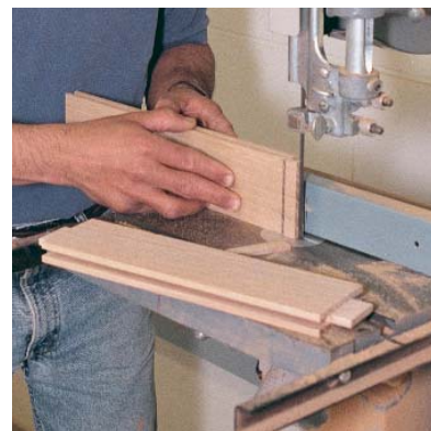
Stub tenons make it plenty strong. With the shoulders cut on a tablesaw, a bandsaw completes the stub tenons on the ends of the rails and short stiles.
