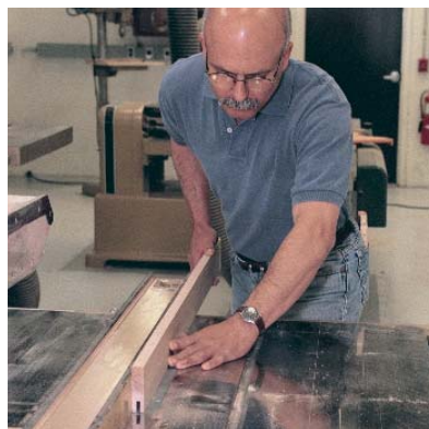
Single groove does double duty. A groove plowed with a dado blade serves as both the mortise for the tenons and the groove to hold the panel.
