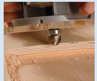
**If you need one, rout the juice groove next.** Use the first template to make an outside template, which will guide a top-bearing, roundnose router bit (top) or a router outfitted with a template guide.
