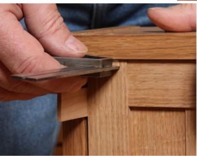
Wedge the door in its closed position. Use a square to determine the proper inset and slip some shims between the case and door to hold it in place for drilling. Use a stop block on the drill to prevent drilling too deep.
