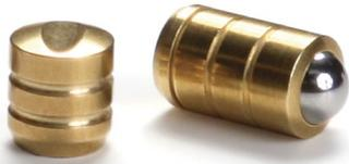
A bullet catch is an elegant and unobtrusive way to keep a cabinet door closed. It consists of two parts—a sleeve with a spring-loaded ball, and a cup that the ball fits into. The trick in installing the catch is to align both parts so that the door closes in the correct position. Here's a simple method.
