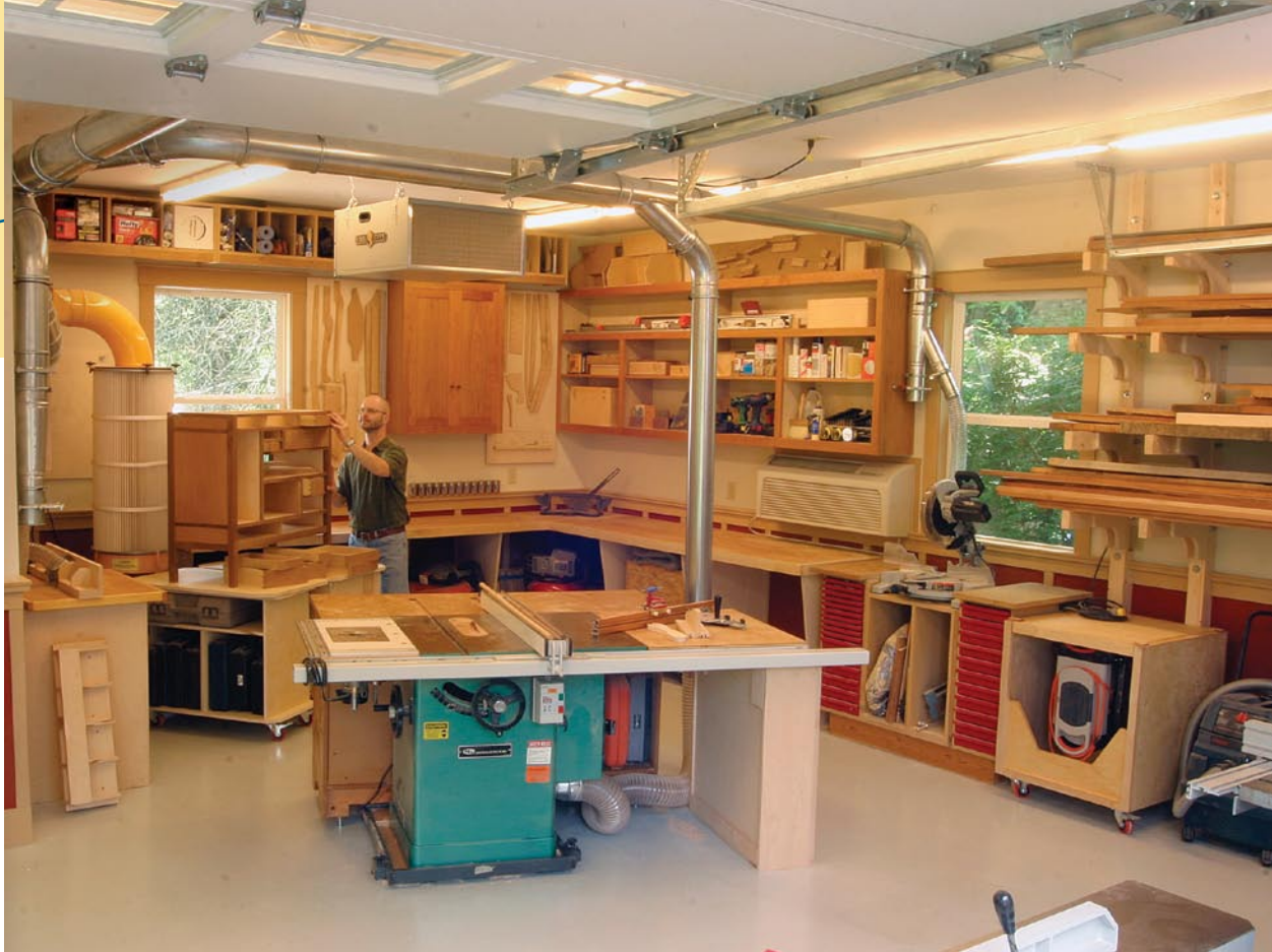
Power central. The larger portion of the shop consolidates the machines and dust-collection ducting, with plenty of lumber storage and all-purpose benchtop space around the outside.
