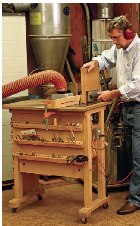
Mobile tools are there when he needs them. When he doesn't, he pushes them against the wall to open up floor space.
