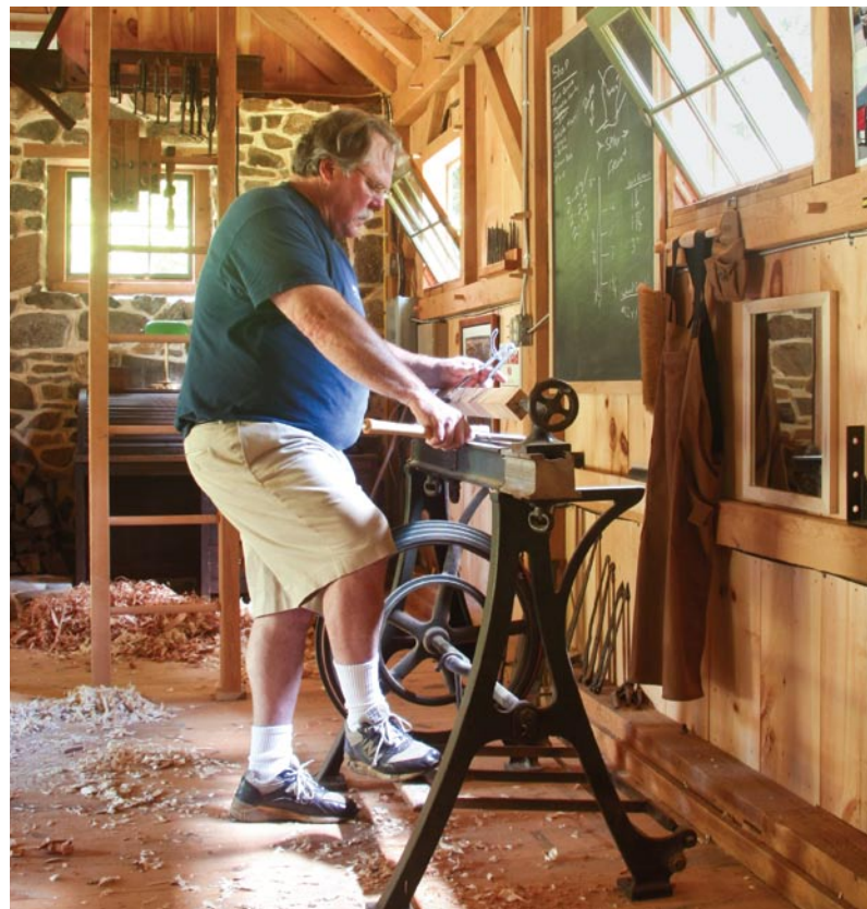
Take the lathe for a spin. Waters likes to make chairs, which need turned parts. A treadle lathe allows him to stay true to his love for traditional, human-powered tools.
