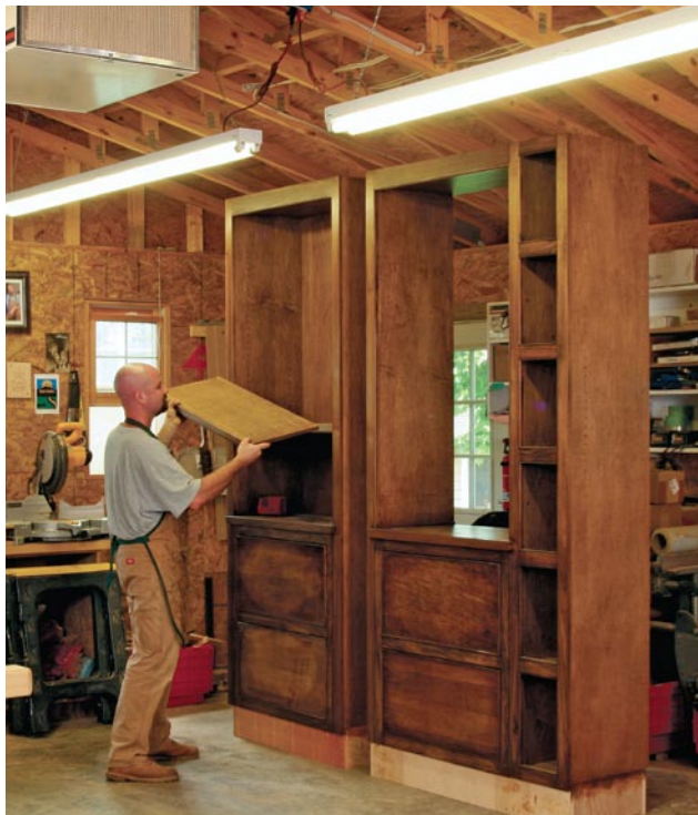
Tall work is no problem. Paolini used scissor trusses on the back half of his shop. The extra height they provide lets him assemble very tall pieces.
