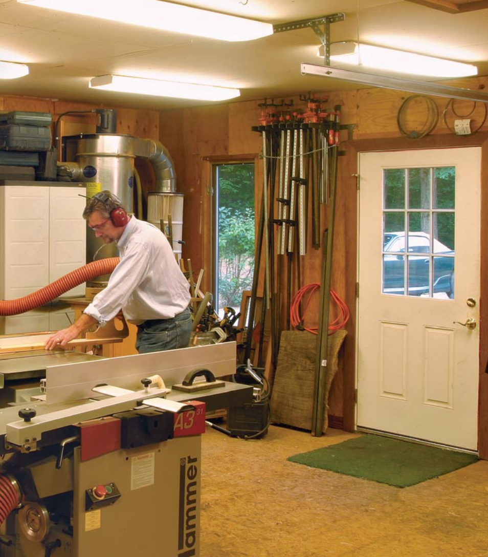
Rolling racks are versatile. To make the most of the shop's wall space, Burkin used inline-skate wheels to create four rolling tool racks. They allow him to use the space in front of the windows without permanently blocking them.
