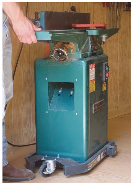
Buy a mobile base. Storing the bandsaw and jointer on mobile bases allows Teague to pull them out into the open when he has to handle especially long stock.
