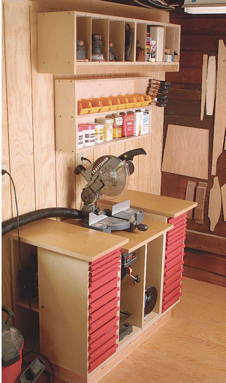
A well-thought-out corner of the shop. The chop saw station not only provides good outfeed support for the saw, but it also stores the grinder and the drill press and houses two banks of drawers.
