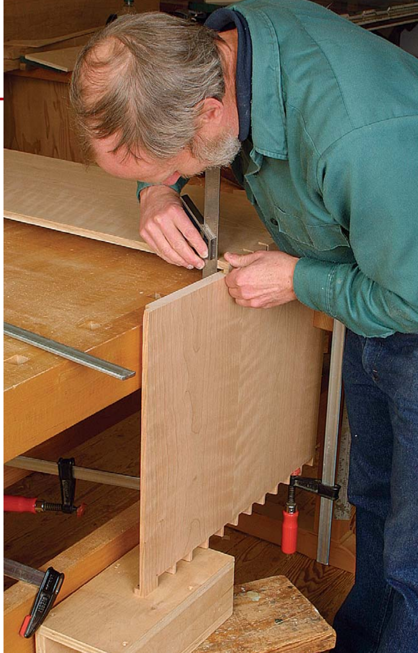
Line up the boards. Before laying out the pins, ensure that the boards are flat and meet at 90°.
