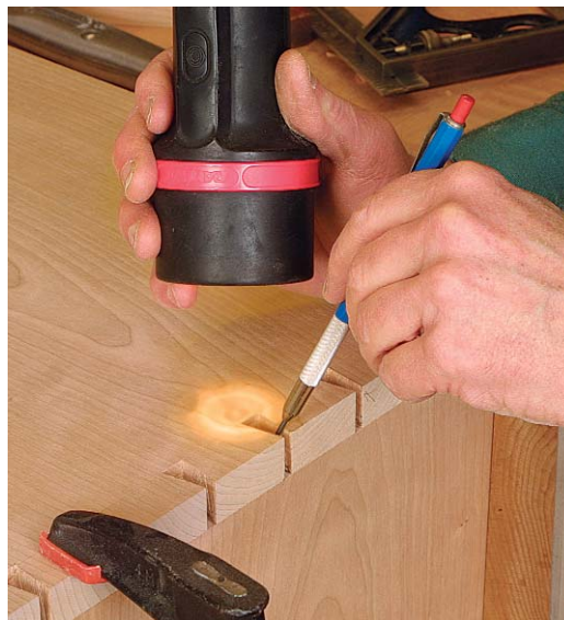
Mark the pins from the tails. With the boards secure, use a sharp pencil to transfer the location of the pins. A flashlight helps you see into the corners.
