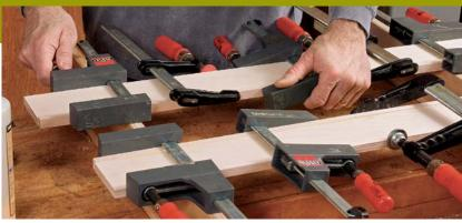
Built to last. Hardwood edging gives the router's guide bushing a longwearing surface to ride on. Edge-glue the strip in place and sand it flush.
