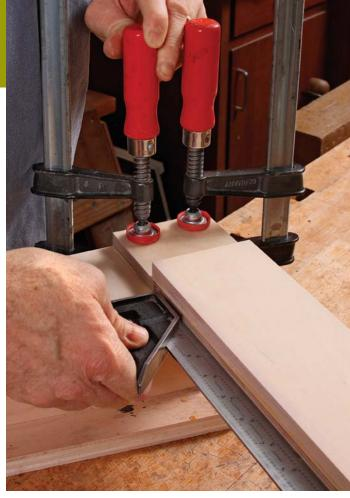
Attach the top of the fence. The top plate of the fence is only there to support the router at the beginning of the cut.
