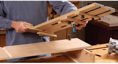
The clamps are underneath, to stay out of the router's way, so you have to elevate the workpiece. But after that the jig is foolproof: You use one of your actual shelves to adjust it for a perfect-fitting dado.
