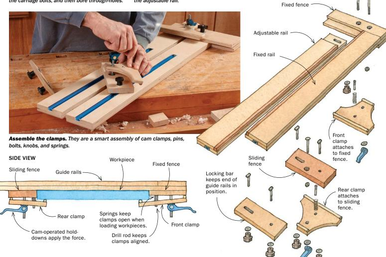
workpiece. Now use the cam clamps and the other fasteners on the fixed and sliding fences to lock the workpiece in place and hold it snug to the bottoms of the rails.
