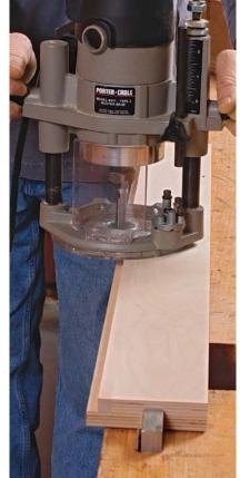
Custom tailoring. Trim the bottom layer of the rails with the same bit and bushing you'll use to cut dadoes. A smooth, straight cut is critical, so be careful not to tip the router.
