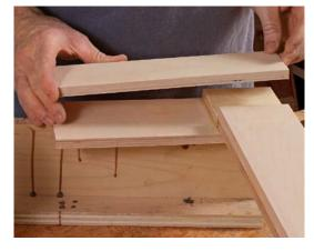
The top should be flush. Use the same plywood for the top surfaces of both the fixed fence and fixed rail. This ensures smooth travel for the router and no unwanted variations in the cut.
