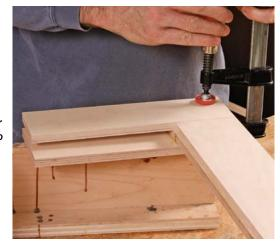
steps. Apply the glue and lightly clamp each fence plate in place with a single clamp. After checking for square, use more clamps to apply greater pressure.
