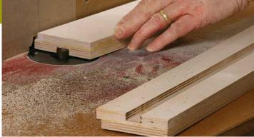
Put tracks under the rails. Rout a ¾-in.-wide stopped groove on the underside of each rail (above), then square up the ends of the groove with a chisel (right). Mount a length of T-track (below) for securing the sliding clamp and locking bar.
