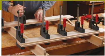
**Offset layers make up the rails.** Leave the bottom layer wide at this point. Alignment is not super-critical, as you will be trimming the bottom rail with the router afterward (see lower right photo).
