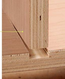
Clamp and go. The cam clamps lock the jig in place quickly, and it's easy to ride each rail for a perfect-fitting dado every time!
