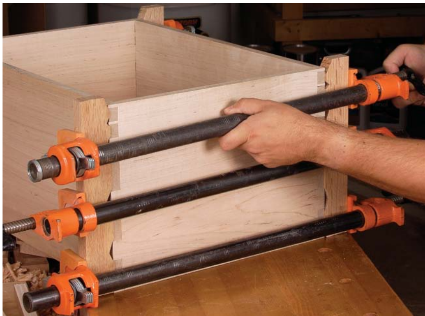
Tight tails. The shaped cauls fit over the pins and apply force to the tails only.
