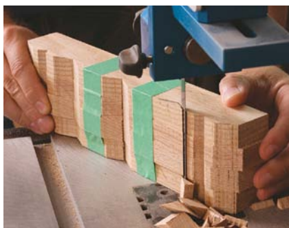
Tight tails. The shaped cauls fit over the pins and apply force to the tails only.
