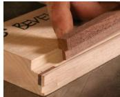
**Grip it and rip it.** Glue a shim into the groove (above) to keep the stock from slipping. Angle the blade at 75° and set the fence so the top of the cut meets the edge of the sled (right).
