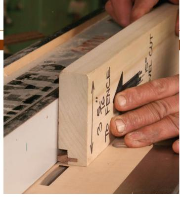
Switch back to the dado set. Extending the rabbet on one side lets the perimeter molding mate with the inside edge of the door frame. Set the dado set for a cut that is 1/4 in. wide by 1/8 in. deep.
