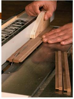
**Start with wide stock.** Bury a dado set in a sacrificial fence (left) to mill a pair of rabbets on each edge. Screw on a hold-down to press the stock tight to the saw table, producing a muntin tongue exactly ½ in. thick. After rabbeting, rip the stock into two ¾-in.-wide strips (above). Be sure to use a splitter and a push stick to control the stock.
