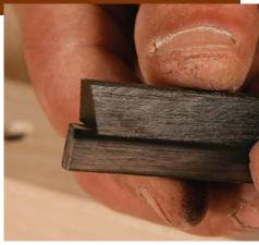
A dovetail bit cuts the cope. Bury the bit in a sacrificial fence. Keep the workpiece tight against the fence and check the bit height with test cuts (left). To help ensure that the top of the muntin lies flush with its neighbor, the bit should leave a tissue-thin layer of waste material (right) that can be trimmed by hand.
