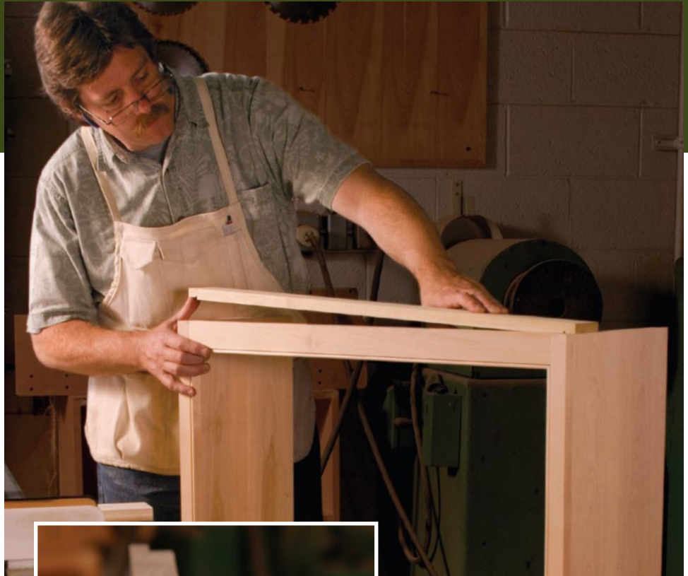
Shoulders first. Working again with the rest of the case dry-fitted, Latta can cut the shoulders accurately. He removes material in small increments from both ends until the shoulders drop snugly between the case sides.
