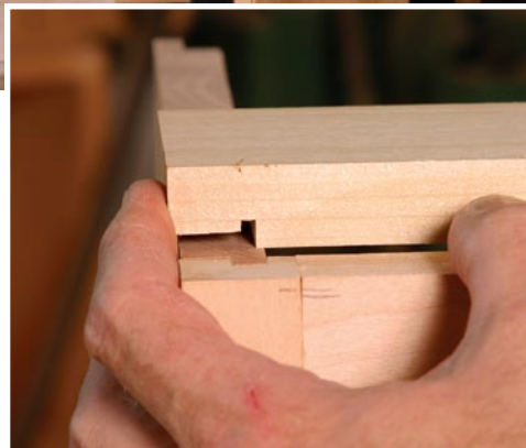
Shoulders first. Working again with the rest of the case dry-fitted, Latta can cut the shoulders accurately. He removes material in small increments from both ends until the shoulders drop snugly between the case sides.
