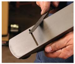
**Soften the edges.** After flattening the sole, ease the corners with a mill bastard file.
