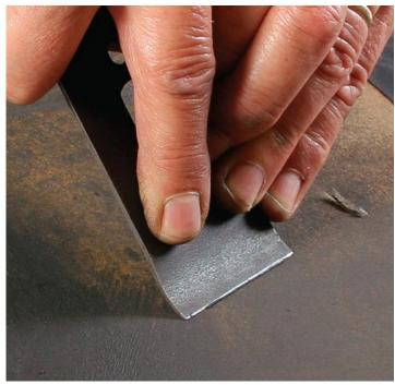
**Smooth the curve.** Polishing the top front of the chipbreaker helps chips slide by smoothly.
