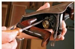
to perfection. When reassembling the blade and the chipbreaker, set the chipbreaker about  $\frac{1}{16}$  in. or less from the tip of the blade.
