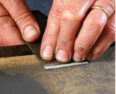
Mind the gap. Any gaps between the chipbreaker and blade (left) will catch and jam chips. Holding the chipbreaker so that its end is below the tip, rub the bottom of the front edge on 220-grit sandpaper adhered to a flat surface (above). The goal is a knife edge that meets the back of the blade all the way across (right).
