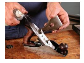
shape, you may have to start with coarser paper. To check your progress, put the blade and chipbreaker together and hold the assembly in front of a white sheet of paper or light background. Look for any gaps between the blade and chipbreaker; keep working until they are gone.
