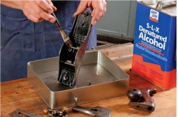
**Follow with an alcohol bath.** Soak and scrub all the parts in denatured alcohol. Dry and then lubricate threaded parts with camellia oil.
