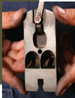
A flat frog is a good frog. Flatten the area from the levercap screw to the bottom. Johnson starts with 120-grit paper glued to a granite plate with spray adhesive. He works through to 220 grit until all the high spots are removed.
