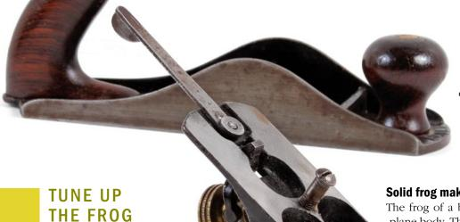
by dismantling the plane. If the plane is rusty, slather on some naval jelly (Amazon.com), a rust-removal product. Then give all the parts a thorough washing and scrubbing in denatured alcohol. Let them dry, and then coat them with a light oil such as camellia oil.
