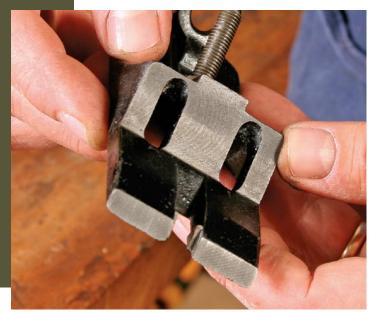
**Grind until it shines.** Check your progress as you go. You're finished lapping when an even rub pattern shows on all the contact points.
