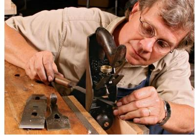
Remedy for a rough throat. If the throat has small nicks, dress the edges carefully with a mill bastard file. Be sure to hold the file perpendicular to the sole.
