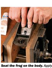
Seat the frog on the body. Apply valve-grinding compound to the four mating surfaces where the frog meets the body (left). Rub the frog fore and aft (above).
