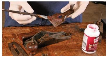
**Naval jelly sinks rust.** Be sure to get it into crevices and even threaded areas. Let it sit for 10 to 15 minutes, then rinse off the parts in water.
