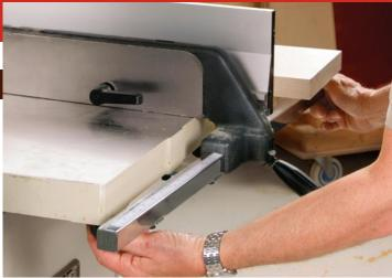
**Get my drift?** With star knobs holding a thick bar that turns on a pivot, both Grizzly machines make it easy to angle the fence to correct for drift.
