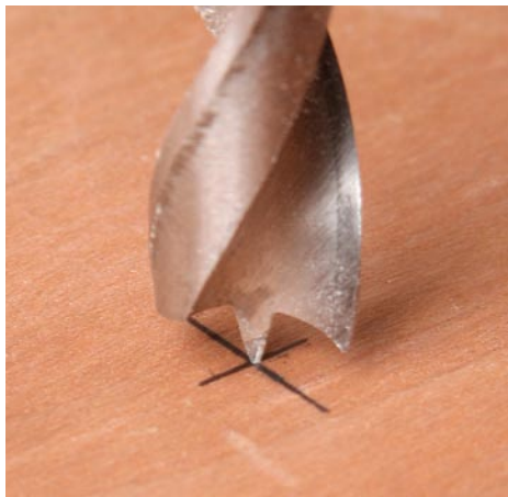
Get a set of brad-point bits. Brad-points center easily on a mark, tend not to wander, and will handle most of your drilling tasks in wood.
