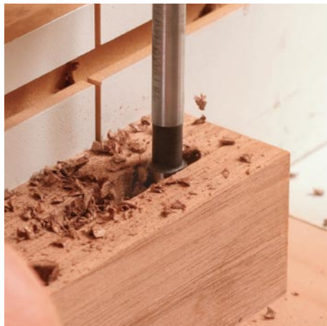
Fun with Forstners. With the drill press's control over location and depth, it's an ideal setup for mortising with a Forstner bit, which can drill partial or overlapping holes (left) without wandering. The drill press also handles large Forstner bits, making it easy to drill holes as large as 2½ in. diameter. The hole's flat bottom makes it ideal for applications like this hardware mortise (right).
