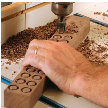
How to use a plug cutter. Use a thick board so the cutter doesn't go through (left). Then use the bandsaw (right) to free the plugs. A piece of tape keeps the plugs on the table.
