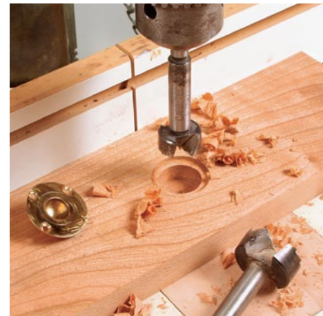
Fun with Forstners. With the drill press's control over location and depth, it's an ideal setup for mortising with a Forstner bit, which can drill partial or overlapping holes (left) without wandering. The drill press also handles large Forstner bits, making it easy to drill holes as large as 2½ in. diameter. The hole's flat bottom makes it ideal for applications like this hardware mortise (right).
