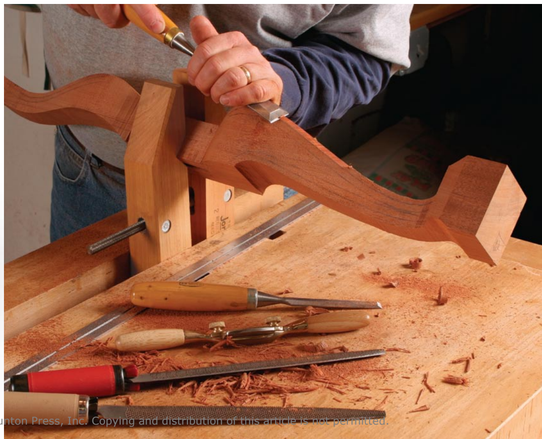
Cabrioles, back to back. The back and side legs are really two cabriole legs in one separated by a square post in the middle. Careful bandsawing now (left) will reduce hand shaping later (below). Chisels, rasps, files, and spokeshaves can all be employed to bring the cabriole legs to their final shape.
