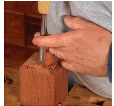
Round the tenons. Guided by a drilled template, round the square tenons using chisels and carving gouges.
