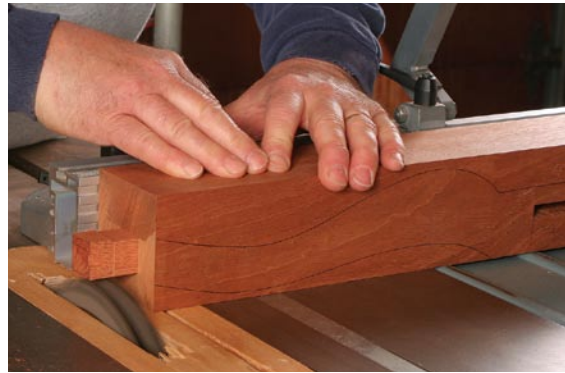
Cut the leg tenons using a dado set. While the leg blanks are still square, cut the tenons on the tops of the side and back legs that connect them to the arm rails.
