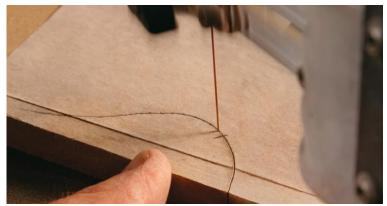
Cut the pattern on the scrollsaw. Glue the tracing to the MDF and score the centerline with a knife. After cutting the pattern and smoothing it with files and sandpaper, carry the layout lines down the edges to the bottom of the pattern.
