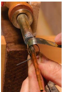
**Shape the stringing.** Latta coaxes a curve into the stringing by bending the pieces over a heated burn-in knife. He uses an automotive feeler gauge as a bending strap to stop the stringing from catching.
