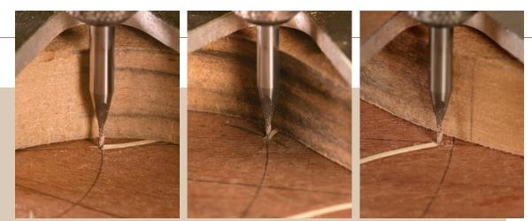
At the leaf's base (left), check to see that the bit starts on the central circle and completely overlaps the existing line of stringing. Where it meets the background leaf (center), the bit should rest on the reference arc and clip the end of the existing stringing. At the petal's tip (right), it should clip the existing line but not go beyond it.
