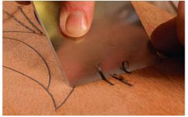
**Give the bird a perch.** Latta uses a separate pattern (top) to rout the simple arcs that anchor the bird design. Leaving the stringing above the surface lets you level it with a smoothing plane iron, used bevel down (above).
