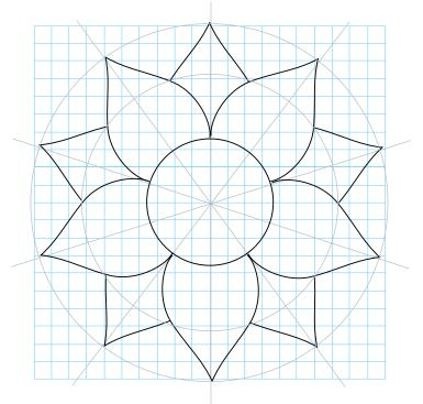
The lotus design, with its repeating complex curves, is tailormade for pattern-routed grooves. The pattern that creates the flower's center is simply a hole drilled with a Forstner bit. The leaf pattern, which creates one half of a single leaf, is sawn into the edge of the same MDF template. To make the pattern, it helps to have a full-scale drawing of the design from which to trace. You can either copy the one shown here or draw your own.
