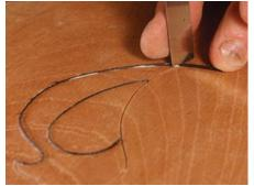
**Apply glue like a surgeon.** Latta uses a syringe with a narrow, curved tip (\$2.60 at leevalley.com) to lay a fine bead of yellow glue into the groove (top). Press the inlay into the groove with your fingers, leaving it just proud of the surface. Trim each end at an angle (above) so the pieces mate cleanly.
