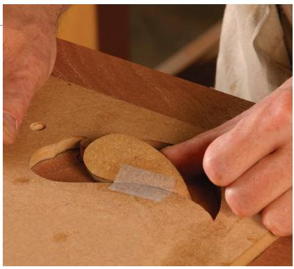
**Rout the wing.** With the perimeter of the body cut, put the wing back in, hold it in place with tape, and rout around it. Avoid thick tape—you don't want the router base hanging up on it. Transparent household tape is fine.
