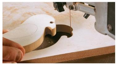
**Make a pattern to guide the router.** Glue the drawing to a piece of MDF and cut out the interior and wing with a scrollsaw (above). Smooth the curves with sandpaper or small files, keeping the edges square to the face. When routing the grooves (right), angle the router and pivot down to start the cut, keeping the bit shank against the template.
