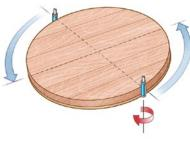
With template and workpiece flipped, the two remaining quarters can now be trimmed cleanly.
