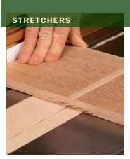
**Cut the dado with a standardkerf blade.** That way you can sneak up on the final width, testing how well the long stretcher fits into it as you go.
