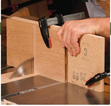
**Start the slot at the tablesaw.** With the blade as high as possible, cut the sides to line up with the dado, and nibble away the waste in between.
