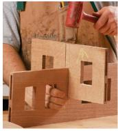
**Start with the stretchers.** As the core of the table, these should fit snugly and squarely.
