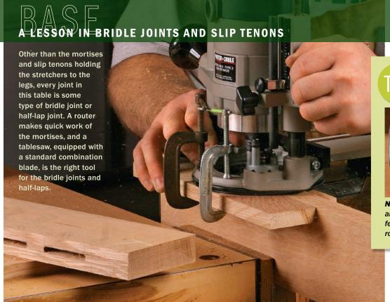
**Rout mortises in the legs.** Use a spiral bit that matches the mortise's width, and use a fence on both sides of the router: Set up the router's edge guide and then clamp on a simple shopmade fence. The mating mortises in the stretchers are done the same way.
