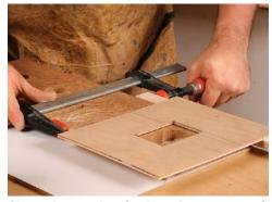
Clamp the template in place. Remove most of the waste in the cutout using a Forstner bit. Then clamp the template to the stretcher. Place scrap beneath the stretcher to protect your bench.
