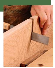
**Go deeper with a handsaw.** Follow the sides of the slot with the saw and then remove the rest of the waste with a chisel.
