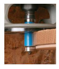
**Always rout downhill.** If you try to rout the whole circle in one pass, you'll tear out the grain in some areas. So you'll need to flip the workpiece. Use a double-bearing, flush-trimming bit so there's no need to change bits or re-attach the template on the other side. Just adjust the bit height to use the other bearing.
