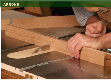
**Slot the aprons and test the fit.** After marking the joint, cut each side first and then nibble away the waste one pass at a time (above). Cut the slots a bit tight at first, and then sneak up on a tight joint, checking the fit (right) after each trimming cut.
