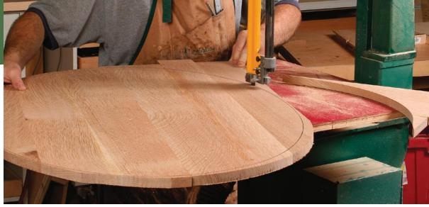
**Cut the top and shelf at the bandsaw.** Use the patterns to trace the shapes. When bandsawing, leave about  $\frac{1}{8}$  in. of waste for the next step: routing the edges flush to your template.
