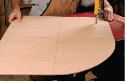
**Cut the pattern at the bandsaw.** Cut just outside the line, so there is less waste to remove when smoothing the curves.
