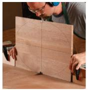
Notch the shelf before cutting the ellipse. Because its width is critical, cut each side of the notch first and then remove the middle. Use stop blocks on your crosscut sled to ensure that notches on opposite sides will line up.
