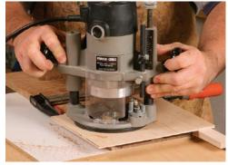
**Trim flush in three passes.** Set the bit depth to  $\frac{1}{4}$  in. for the first pass,  $\frac{1}{2}$  in. for the second, and  $\frac{1}{8}$  in. on the last one.
