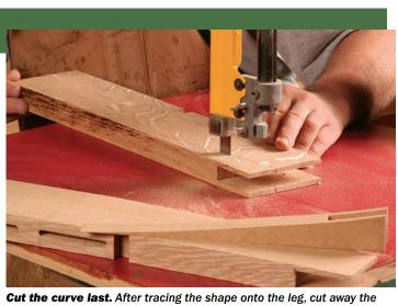
**Cut the curve last.** After tracing the shape onto the leg, cut away the waste on the bandsaw, and then clean up the saw marks with a handplane or sander.
