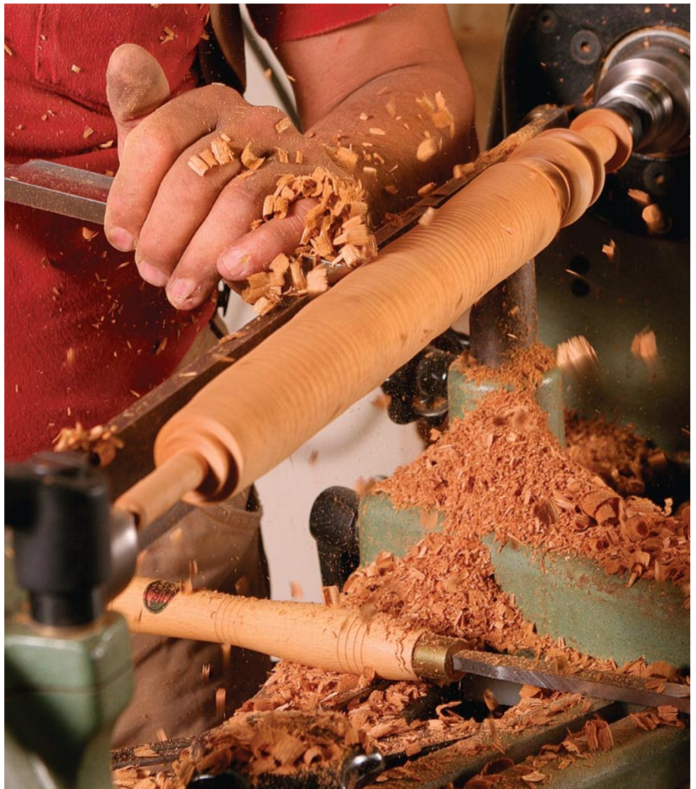
Get ready for reeding. Turn the details at the top of this post. Then use a spindle gouge to cut a straight taper, from 1 5/8 in. dia. to 7/8 in.
