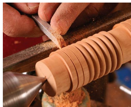
A shopmade fixture holds the work. The workpiece mounts on a mandrel turned to fit snugly in the mortise. The mandrel is held in a chuck. The opposite end of the workpiece is held with a live center in the tail stock.
