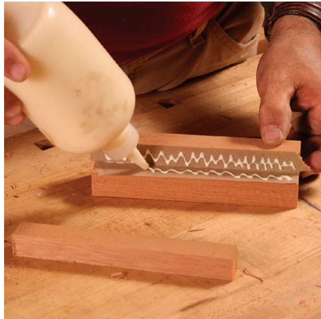
Notch the blank. Cut away one quarter of the leg. Then, to make the blank whole for turning, glue in a piece of scrap. A layer of kraft paper makes the scrap block easy to remove later.
