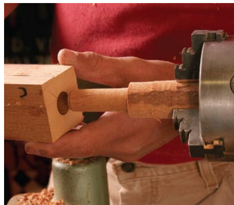
Notch the blank. Cut away one quarter of the leg. Then, to make the blank whole for turning, glue in a piece of scrap. A layer of kraft paper makes the scrap block easy to remove later.
