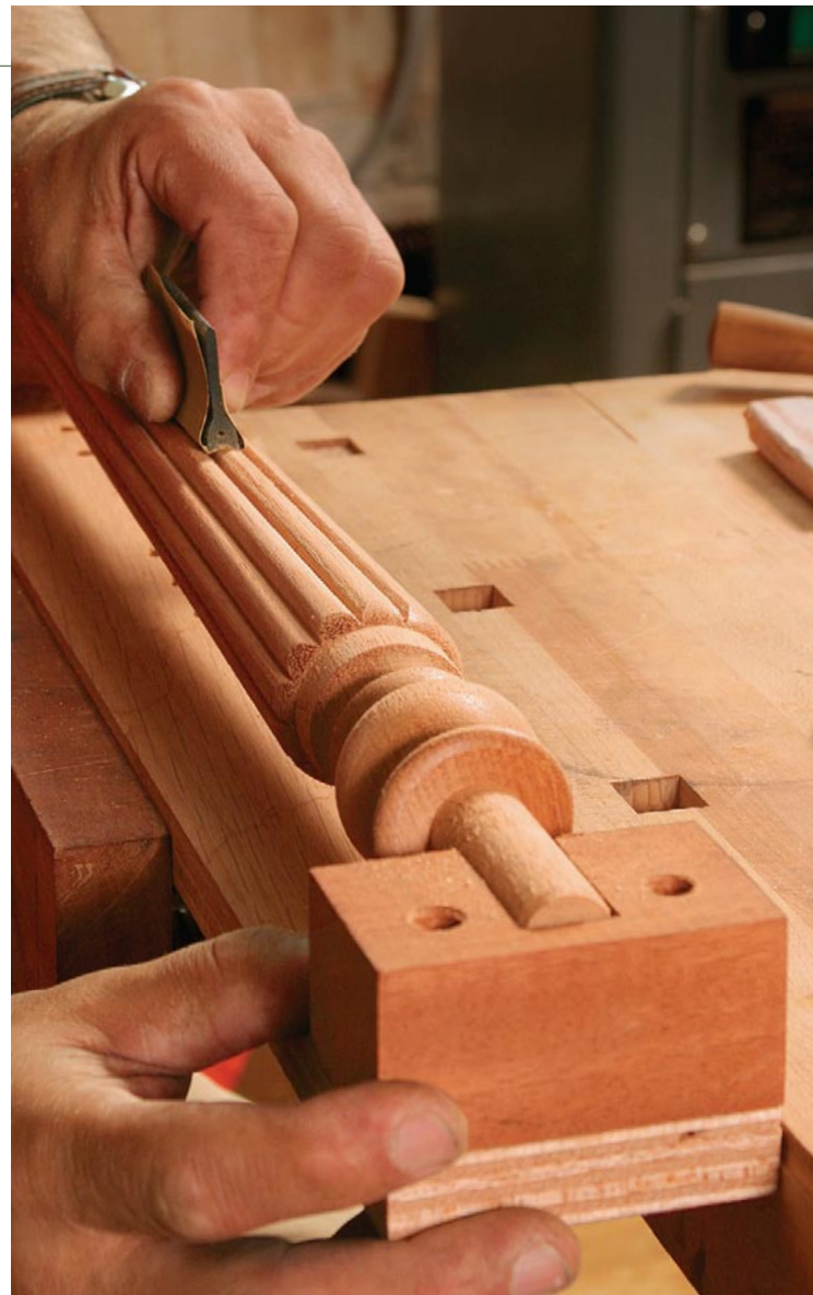
Shaping the reeds. Rodriguez mounts the workpiece in a shopmade jig, then uses a variety of tools to round the tops of the reeds and sharpen the grooves.
