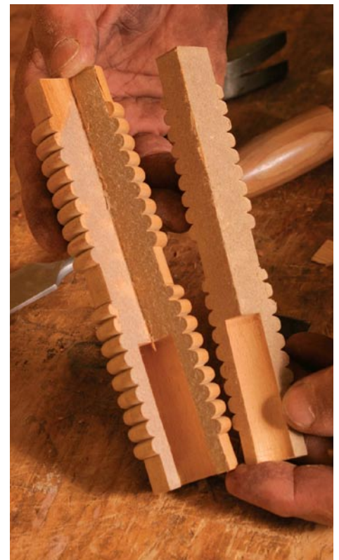
Turn the rings with a bead-cutting tool. Use the tool to score the outline for all of the rings as a reference before forming them. Afterward, use a sharp chisel to pry away the glued-in filler block.
