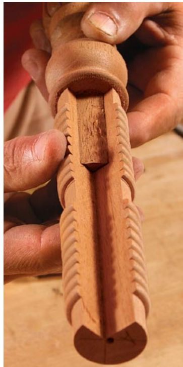
Create a flat on the tenon. The tenon will be exposed by the cut-away portion of the leg. The flat surface lets the legs marry to the beveled corners of the case.
