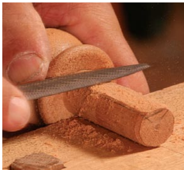
Create a flat on the tenon. The tenon will be exposed by the cut-away portion of the leg. The flat surface lets the legs marry to the beveled corners of the case.
