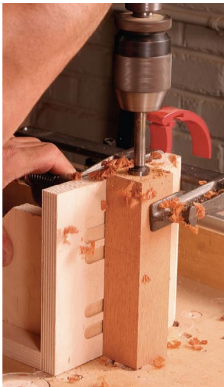
Drill a round mortise. Clamp a right-angle jig to the drill-press table. This helps ensure that the mortise runs straight.
