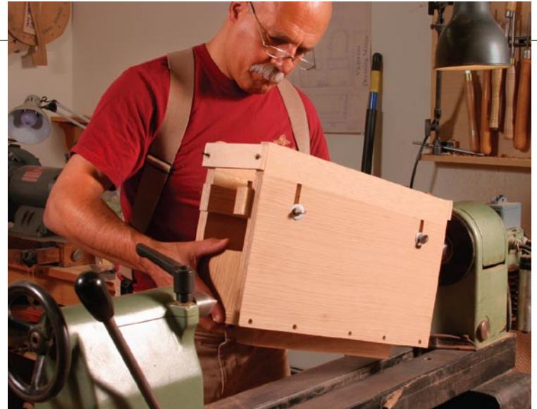
A box for reeding. Before mounting the workpiece between the lathe centers, Rodriguez clamps the reeding jig to the lathe bed.
