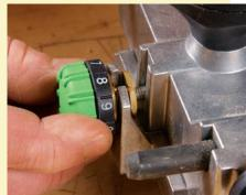
Festool's micro-adjust knob is even better. The fence is captured on the screw so that it moves both in and out with adjustments, and the knob is graduated.
