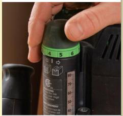
Festool offers very fine microadjustments. The numbered and audible detents on the knob are separated by 0.1 mm.
