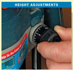
Height adjustments are easy on the Bosch. Loosen the lock and twist the knob. The depth rod raises and lowers on a rackand-pinion gear.
