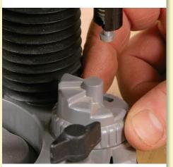
**Bosch's turret has preset stops.** There is ½-in. difference between the six stops. This saves setup time, but can be a bother if your plunge depth isn't a multiple of ½ in.
