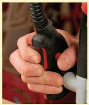
Trigger switches are convenient and safe. Both hands grasp the router when it starts. The Freud (shown here), Festool, Bosch, and Porter-Cable routers all have one.
