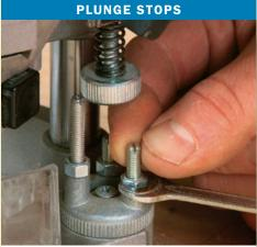
Adjustable plunge stops are more versatile than preset ones. They give precise control over how much material is removed on each pass. All but the Bosch have them.
