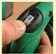
**Two smart ways to adjust speed.** With Hitachi's thumbwheel (left), both hands stay on the handles during speed changes. The Porter-Cable marks speed with RPM (right), so it can be set exactly to a bit's required speed.
