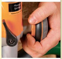
**Triton offers a second way to plunge.** Pull in the orange lock collar and twist the handle to lower the body on a rack-and-pinion gear. It's a nice way to get precise plunge control.
