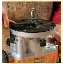
Bit changes are easiest on the Triton. The spindle locks automatically. That frees up one hand to hold the router body for more stability.
