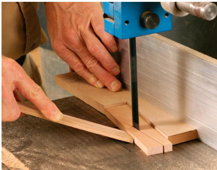
Bandsaw is safer than tablesaw. Rogowski uses a simple jig made of \frac{3}{8} -in. MDF with an 8^\circ notch cut into it.
