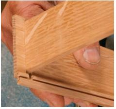
Add the slip after assembly. A small notch toward the rear of the slip accommodates the drawer back, while easing the inside edge produces a clean, finished look. Gluing even the shortest slips will require a surprising number of clamps (right) because the material is thin.
