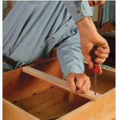
Dovetail the front, notch the back. Hack dovetails the center divider into the front (top). After confirming that the drawer box is square, Hack centers the divider on the drawer back, then glues and screws it in place (bottom).
