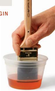
**Dip a toe in.** Only submerge about a third of the filaments in finish. If you go deeper, it is harder to apply an even coat. Also, finish will tend to pool in the bottom of the brush and then run down the ferrule when brushing vertical surfaces.
