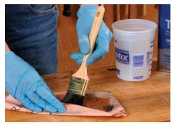
**Solvent, then soap.** Rinse the brush two or three times in mineral spirits, then remove the solvent on newspaper before cleaning the brush with hot water and soap.
