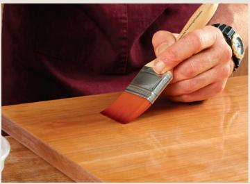
Brushing the last coat. Taklon brushes are ideal for the last, thinned coat of finish. But there is a specially made Taklon brush (right) for waterbased finishes that can't be thinned as much.
