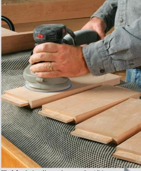
Work in stages. Use each successive grit to remove the scratches left by the last one, until the abrasive is so fine (P220 or more) that the human eye can't see the scratches under a finish.
