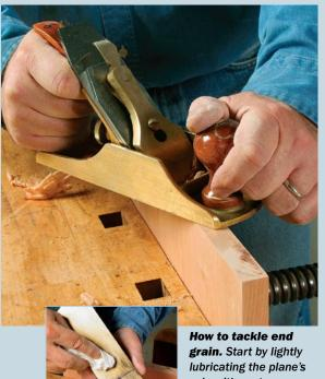
How to tackle end grain. Start by lightly lubricating the plane's sole with paste wax. To avoid chipout at the far edge, take a few short passes from that end first. Then rotate the piece and work normally, stopping short of the far edge.
