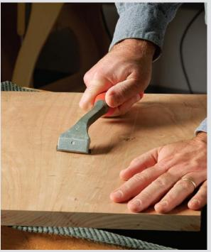
Scrape away the glue first. Christiana starts work on the tabletop by using a sharp paint scraper to remove the glueline in the middle of the panel.
