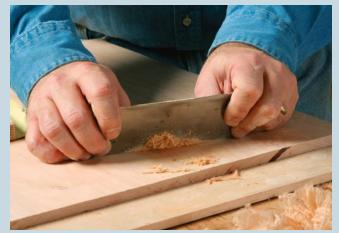
**Treatment for tearout.** Pekovich typically uses a card scraper to remove any tearout.
