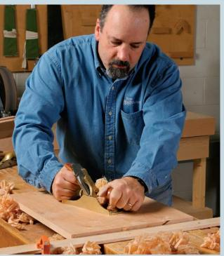
Plane in two stages. First, level any high spots until the top is flat on both sides. After resharpening the iron, set the plane for a light cut and take a series of smoothing passes over the entire surface of the show side only.
