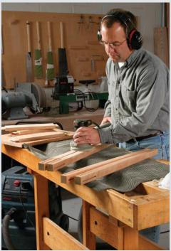
**Gang up parts.** Start with a coarse grit, P80 or P100, to remove burns and mill marks. Avoid rounded edges on narrow stock by ganging two narrow pieces together. Note, this only works if the surfaces are level.
