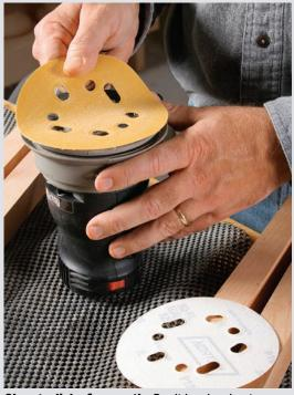
Change disks frequently. Don't be shy about using more than one disk of the same grit before moving to a finer abrasive. A worn or clogged disk will slow down the work.
