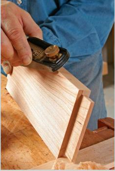
**Don't bother with hidden surfaces.** To save time and wear on the blade, plane only the outside face and bottom edge of each apron. Afterward, chamfer the bottom edges with a block plane.
