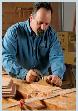
**Easier than benchdogs.** A simple planing stop clamped across the benchtop is all you need to secure the work, and it lets you quickly flip the piece or change to another.
