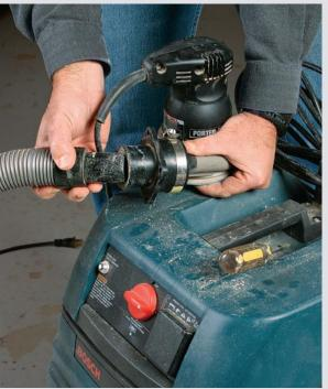
Better than a dust mask. Connect a shop vacuum to the sander's dust port to keep dust out of the air and avoid clogged sanding pads. Better vacuums switch on with the sander when the tool is plugged into an onboard power outlet.
