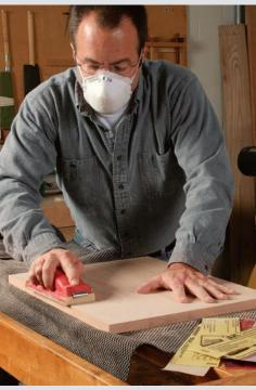
**Finish by hand.** Begin hand-sanding with the last grit you used on the random-orbit sander, usually P220. Work the sanding block in the direction of the grain to remove the last swirl marks from the sander.
