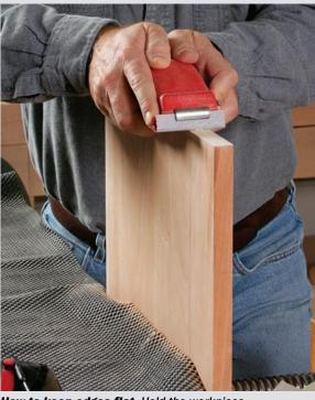
How to keep edges flat. Hold the workpiece in a vise, with the narrow edge horizontal. Use the sanding pad like a block plane, running your fingertips along the workpiece to keep the block flat and the edge square.
