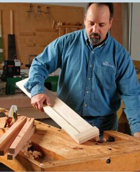
mounts in the vise and holds the leg securely during planing.
