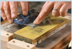
**Get sharp first.** Using waterstones and a honing guide, Pekovich polishes a narrow band at the blade's beveled tip (top). He removes the burr with his finest stone (bottom). For more, see "A Visit to the Sharpening Doctor," FWW #206.
