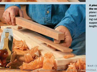
Mark the top end of the taper. Planing too much on the tapered area can cause the intersection with the flat area to move. To avoid this, draw a few pencil lines just below the intersection as a guide.
