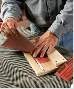
**Shopmade paper cutter.** Christiana's cutting jig uses an old hacksaw blade to trim sandpaper sheets squarely to fit on padded sanding blocks. The blocks hold the paper flat, ensuring that it will leave a flat surface.
