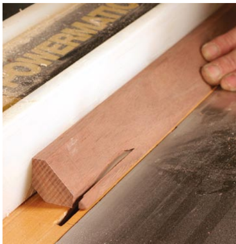
Trim the sides. With the blade set at 90°, cut away the sides of the blanks where they extend above the top of the cradle.
