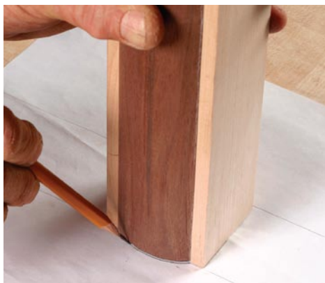
The cradle determines the tool. Use the cradle and the curved quarter-column blank to help lay out the scratch-stock holder.
