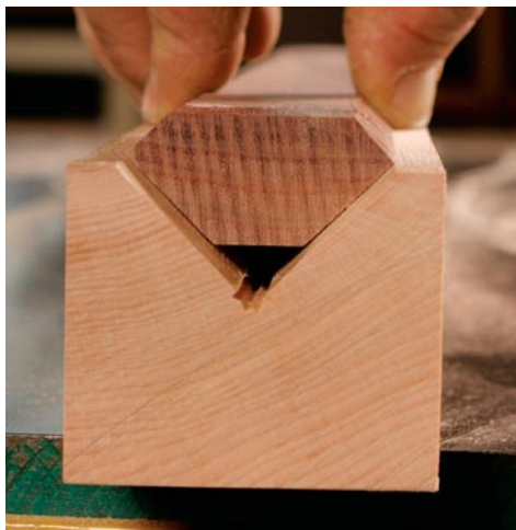
Test the fit. Place the blank in the cradle and check that the sides terminate flush with the cradle's top.
