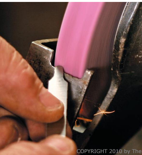
Two profiles on one piece. Start with a piece of card scraper or old hacksaw blade. On one end, grind the rounded profile for scraping the fluting (left). On the other end, grind the concave profile for the beaded stop-fluting (above). Any burr raised is insignificant, and the tool is used in both directions.
