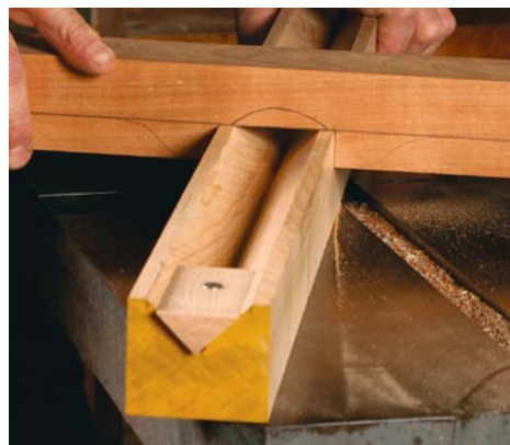
No slop allowed. To cut straight flutes, the cheeks of the scratch-stock holder must fit snugly against the sides of the cradle.
