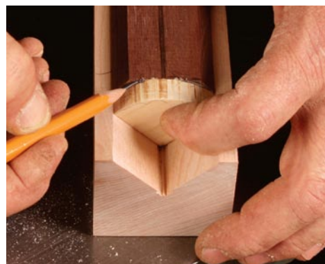
Transfer the shape. Place the template against the end of the blank and mark the desired curve.
