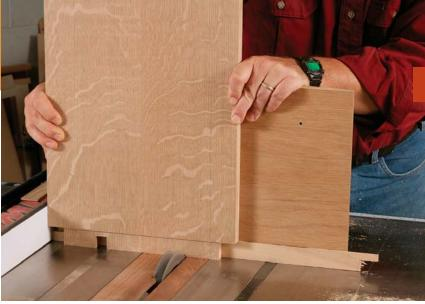
Dado blade does most of the work. After cutting the tenon cheeks and shoulders with a dado set, cut the through-tenons to width, using a tall fence to support the board. The scrapwood behind the tenons backs up the cut and reduces tearout.
