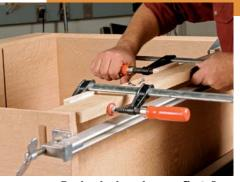
**Backsplash and apron first.** Dryfit the case to ensure proper alignment when gluing the backsplash and apron to the case top and bottom. These parts will help keep the case square in the later stages.
