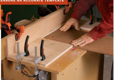
First cuts. Clamp stop blocks on both sides of the bit for the stopped cuts. With the spacer in place (see drawing below), plunge through the template and make one pass in the first mortise slot. Just flip the template to do the opposite slot.
