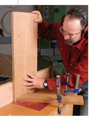
**Rout the dovetail keys.** After cutting the dividers to length, use the dovetail bit to cut the keys. A tall fence supports the long boards and a featherboard keeps the piece snug against the fence.
