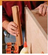
**Top, bottom, and sides.** Use grooved clamping cauls over the through-tenons to get pressure where it's needed (above). Place the case on T-supports to make clamping easier (right). Be sure to keep glue off the ends of the through-tenons.
