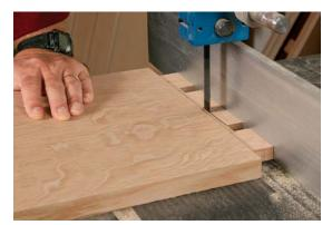
Saw off the stub tenon. Use the bandsaw to cut the stub tenons to length. The fence ensures a parallel cut.
