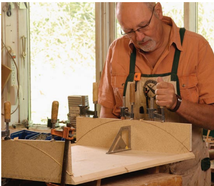
Outer ribs come first. Glued and clamped manually, these prevent the other ribs and spacer blocks from sliding toward the ends of the form.
