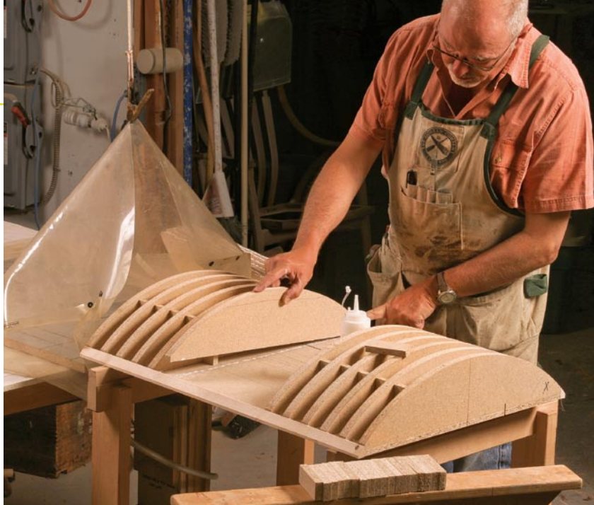
Add the inner ribs. The ribs are 2 in. apart. Spacer blocks hold them perpendicular to the base.
