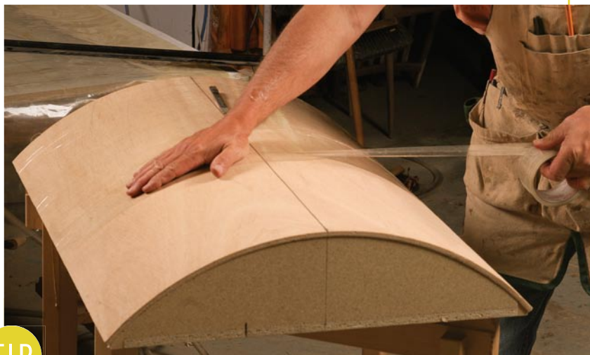
Packing tape keeps the glue off the form. Also, mark a centerline and use it as a reference to align all the plies on the form.
