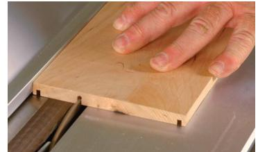
One piece, three grooves. While the sides of the box are one continuous piece, cut grooves for the top and bottom panels, and then cut a third groove that becomes the inside rabbet. Use a rip blade for these cuts; it leaves a square kerf.
