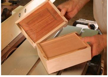
The inside-out box. With the cuts complete, the top and bottom of the box are revealed (left). Sand away the saw marks on the top and bottom edges (below). The rabbets should need very little trimming.
