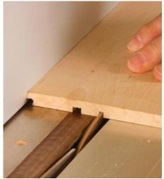
**Cut rabbets and grooves.** Cut the two parts of the rabbet joint on opposite edges of the board (left). Then cut the grooves for the top and bottom panels (right).
