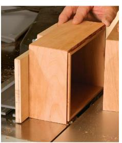
The rabbet revealed. Once the fourth side has been cut, the lid will come away, revealing the two halves of the rabbet joint. Sand or plane the rabbets to clean up the saw marks and fine-tune the fit.
