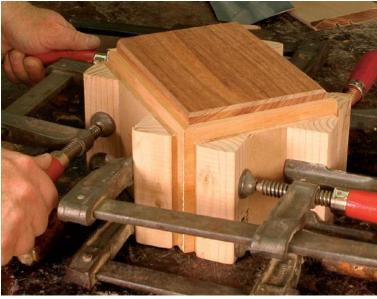
Assemble the box. You can reinforce the miters with biscuits. In any case, apply glue to the mitered ends, place the top and bottom panels in their grooves, and assemble the box (left). Use 45° blocks, glued to ¼-in.-thick MDF, to align the clamping force with the joint. Use light force from clamps resting on the bench to align the cauls with the box sides, and then apply the upper clamps, which are more centered on the joint (above).
