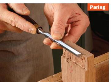
Long blades pare better. Chisels with short blades, such as Japanese-style ones, are not able to pare as wide a joint as the longer-bladed chisels. Plus, there is less blade to hold with the forward hand for fine control.
