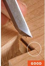
Why side bevels are important. If a chisel's side bevels terminate in large, flat sides, the chisel will not fit into tight corners (left). Chisels with very narrow, flat sides are ideal for getting into dovetails (right).
