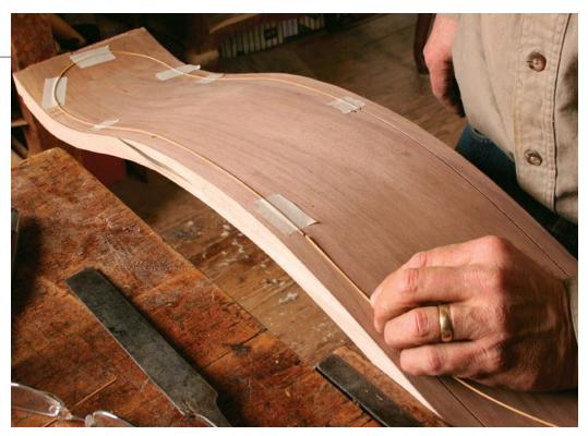
leaving a slot for the fine line. I find it helpful to score a very light line on the inside of the channel using the point of a compass. This gives you something to register the V-channel tool in. Then walk the tool around the circle, giving it a light tap with a mallet at each step. You should aim to create a channel slightly shallower than the thickness of the lining.
