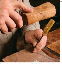
**Punch a curved channel.** Register a modified screwdriver in the compass line, and cut around the curve with a series of sharp taps.
