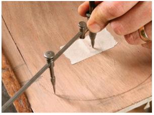
**Compass guide.** With the sharp point of a compass, scribe a very light line along the inside of the circle.
