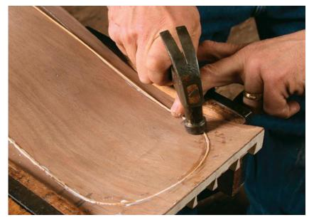
Insert the lining. The channel should be tight enough so that when the lining is pressed in, it requires no clamping. When dry, use a paint scraper or a cabinet scraper to bring the lining flush with the veneer and remove all excess glue.
