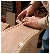
**Dry-fit the line for length.** Fine lining generally comes in yard lengths, so a couple of joints will be required. Cleanly cut joints will be practically invisible once the piece is finished.
