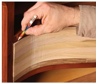
across the width of the core to keep the thickness even. With today's thin veneers, you must be very thorough in cleaning up the core because any ripple will transfer through the veneer.
