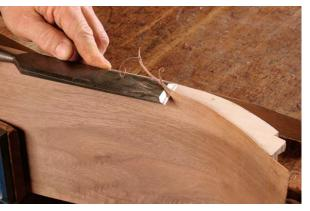
Trim the edge. Use a wide chisel to pare the overhanging veneer flush with the core.
