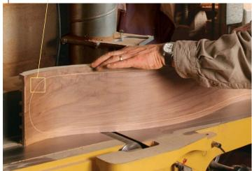
**Reduce the height.** Use a jointer followed by a handplane to reduce the drawer height to the scribed lines for the top and bottom sections of cock beading.
