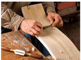
Clean up the bandsaw marks. Use flat and curved spokeshaves to clean up both sides of the core.
