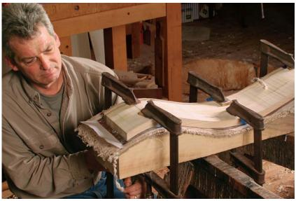
**The core as a caul.** You can use either another serpentine core or the remains of the block from which the cores were bandsawn as a clamping caul.
