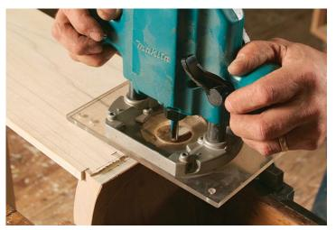
**Assemble the drawer and trim the ends.** Use a straight bit in a router to cut away the ends of the drawer front. Rout close to the scribe line, and finish the job with a chisel.
