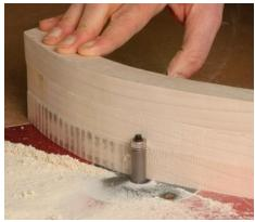
Clean up one at a time. After smoothing one layer, glue a bandsawn layer below it and use a template bit to clean it up. Glue on each successive layer and smooth it with the template bit.
