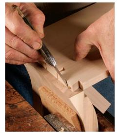
Lay out the pins. Use a piece of wood the thickness of the drawer bottom to align the grooves on the drawer front and side. Mark the location of the pins on the drawer front.
