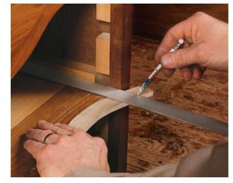
Flush-fit the drawer front. With the drawer front cut to height and width, place it in the opening and mark any areas on the face that need to be trimmed flush with the carcase. Use the spokeshaves to do so.
