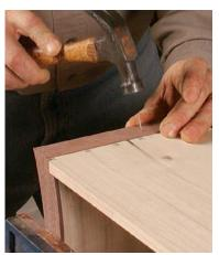
Top and bottom, then sides. Offcuts from shorter drawer cores are used as cauls when clamping the top and bottom sections of cock beading (left). For the side cock beading, because the sides of the drawer front are end grain, reinforce the glue joint by countersinking brads (above).
