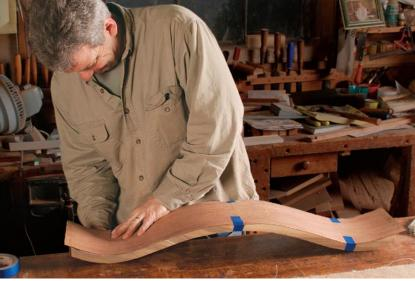
**Align the veneer.** After you apply white glue to the veneer and the core, hold the veneer in place with masking tape to prevent it from shifting when pressure is applied.
