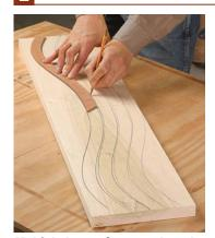
Multiple layers from one board. To bandsaw less wood at once, lay out multiple layers of core on one board and then bandsaw them out.
