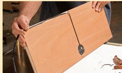
A rabbet continues the path. A rabbet along the back of the shelf carries the wire to a corner, where it can be routed to a transformer or multi-tap connector.
