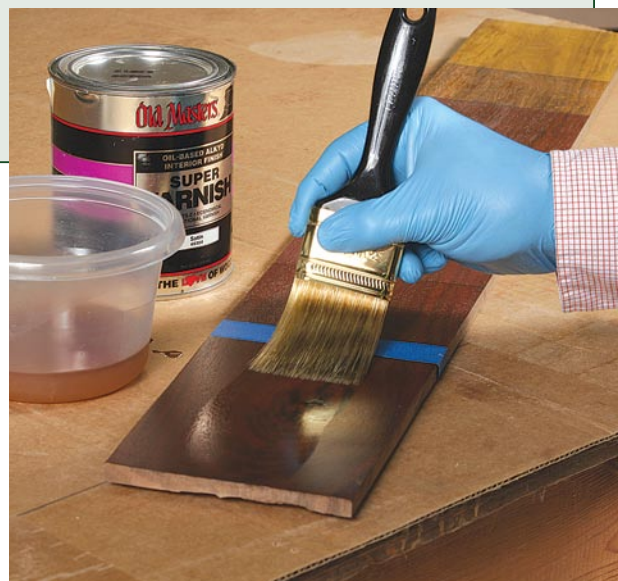
From prep to finish. Start by scraping, planing, or sanding the sample board as you will the actual workpiece (left). Then mark the lines separating each step in the coloring process (center). Then apply the finish, coat by coat, until the desired color and gloss are achieved (right). A piece of blue tape offers a way to isolate a section.
