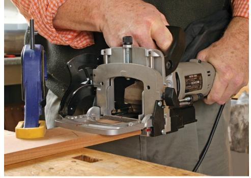
**Center the cutter on the stock's thickness.** With the fence flat on the workpiece, adjust its height to locate the cut. To make the cut, simply align the joiner with the single layout mark, start the tool, and push the joiner's body forward.
