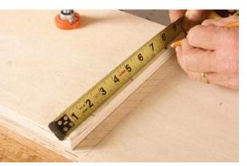
**Layout trick.** To start, mark out the shelf location on the case side and clamp the actual shelf along one of those lines. You are now set up to cut both sides of the biscuit joint.
