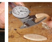
**Simple and efficient.** An adjustable stop on the joiner (left) controls the depth of cut to match each of the common biscuit sizes—0, 10, and 20. A biscuit swells in thickness (right) when wet glue hits it, helping to anchor the joint. So store biscuits in a sealed jar to keep out moisture.
