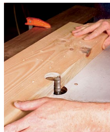
Push the fence into the bit. The infeed edge of the bit is buried, so the workpiece fibers are fully supported where the bit exits the cut.
