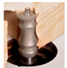
Push the fence into the bit. The infeed edge of the bit is buried, so the workpiece fibers are fully supported where the bit exits the cut.
