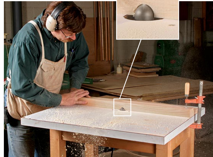
Bury the bit. Clamp one end of a wooden fence to the router table and, from the other end, carefully pivot the fence into the rotating bit. Then clamp it down.
