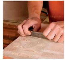
**Good preparation is key.** To avoid tearout, smooth the figured maple with a scraper rather than a handplane. If you sand, vacuum the dust thoroughly.
