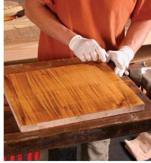
An overall tone is the final color. After sanding away most of the second dye, apply a coat of yellow dye to give the whole piece a warm or antique look.
