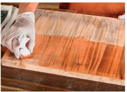
Warm up the figure. Apply red or dark amber to add a subtle secondary color to the figure, which will be revealed when the piece is clear-coated later.
