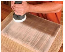
Sand back to mostly bare wood. Use P220-grit sandpaper to remove most of the dye, leaving darker stripes in the end-grain figure, where the dye was able to penetrate deeply.
