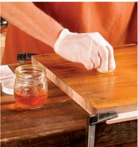
To bring out the huge curl and deep figure in the maple, apply a thin coat of walnut or boiled linseed oil. Add a few drops of oil to a pad and very gently coat the entire surface you are working on. Then wipe it off with a clean cloth. This brings out the wood's depth and luminosity, making the grain appear to move as your perspective changes.
