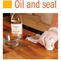
Pop the curl. Rub in a very thin coat of a drying oil to bring out the threedimensional shimmer of the maple's figure (above). Then apply a thin, clear, glossy topcoat such as shellac (right).
