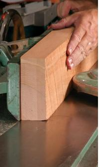
**Joint an edge.** Register the freshly jointed face against the fence (left) and again take light passes until the edge is flat. If the fence is set at 90° to the jointer table, the two jointed surfaces should now be square to one another.
