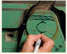
**Grain matters.** To reduce tearout, consider the rotation of the cutterhead and the direction of the grain when deciding which way to feed a board. Fortune marks his jointer near the cutterhead for easy reference. The diagonal lines represent proper grain orientation.
