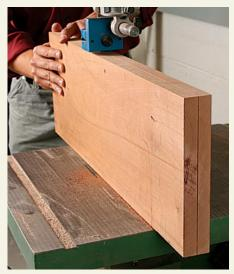
**Taking a heavy resaw cut.** It's also possible to resaw to yield two or more boards from one piece of stock.
