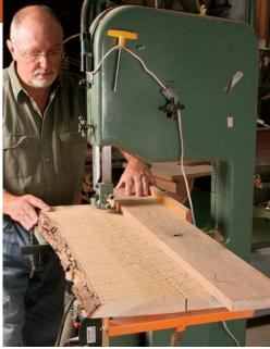
**Rip without resistance.** Fortune sets up his bandsaw with a coarse, 3-tpi, skip-tooth blade, tracked on the centerline of the upper wheel. This makes it easy to cut thick stock. Boards without a straight reference edge can be ripped freehand (left). Or use a straight-line jig (right) to guide the stock through the blade.
