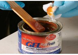
**One thick finish.** The easiest way to control how much gel varnish goes onto the cloth is to place it on with a stirring stick.
