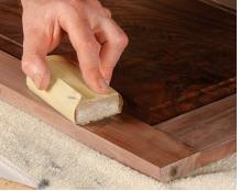
Seal the surface. Wipe the cloth over the surface no more than a couple of times to leave a thin film of shellac on the wood (above). Use P320-grit sandpaper wrapped around a sanding block to smooth the surface (left). Remove the dust with a vacuum or compressed air.
