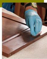
Apply dark wax directly. If you want dark wax to enter the pores to change the tone of a piece, wipe the cloth into the wax (left). Work it into the wood and then wipe with the grain to remove the surplus (right). Buff the wax, clear or dark, until the surface is silky to the touch (below).
