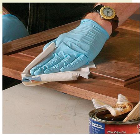
Rub on the gel varnish, then wipe off the surplus. Work the finish into the wood using small, circular movements, then wipe with the grain to remove any thicker deposits (left). Don't try to cover too large an area or the finish will become tacky before you can buff it. Use a clean cotton cloth to wipe away the surplus gel varnish (above), turning the cloth frequently to keep exposing a clean surface.
