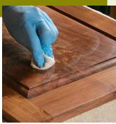
A thin film of wax. Fold over a piece of cheesecloth a couple of times and then place a lump of paste wax in the center (left). Gather the corners of the applicator and then press down until the wax begins to ease out through the rounded face of the applicator. To avoid having light wax show up in the pores of dark wood, use light pressure on the applicator.
