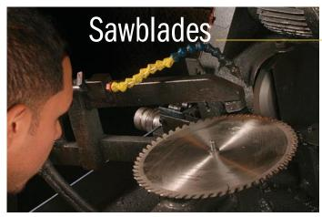
Sharpening at the shop. Professional sharpening services have the specialized equipment and know-how to turn dull bits and blades into sharpones (above). Most sharpening services also can replace chipped or broken carbide teeth (right).
