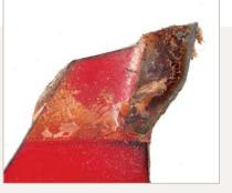
Resin is double trouble. Resin buildup on carbide teeth creates corrosion and extra heat, and both are bad
