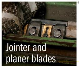
Dull no more. A grinding wheel passes along the cutting edge of a jointer knife, leaving behind a sharp, nick-free surface.
